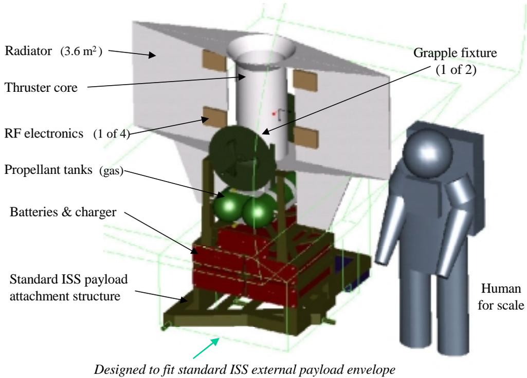
Figure 2: Preliminary design of VASIMR Experiment for the International Space Station
