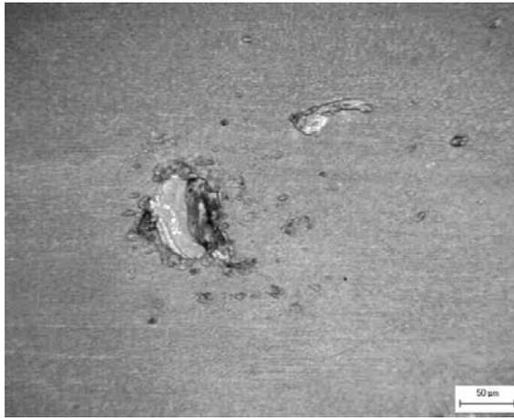
*Fig.5 Scratches and craters on the solar elements surface for the group B<sub>3</sub>*
