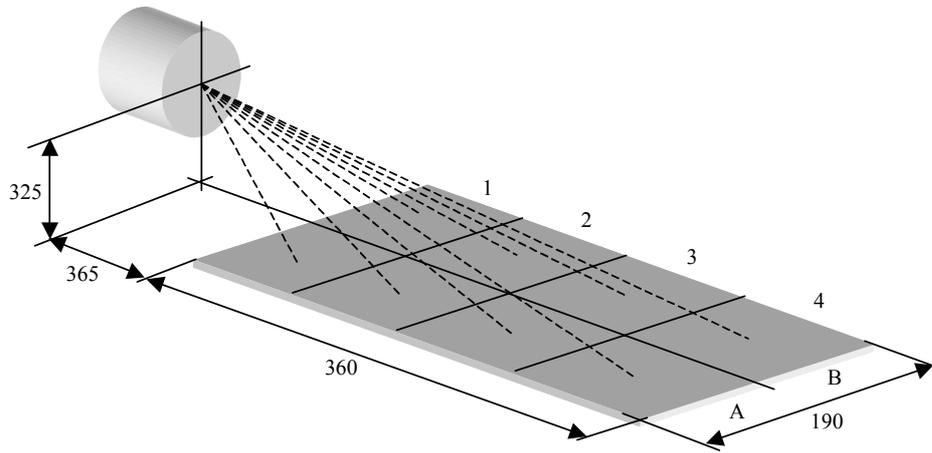
Figure 1: Thruster and SB segment disposition
