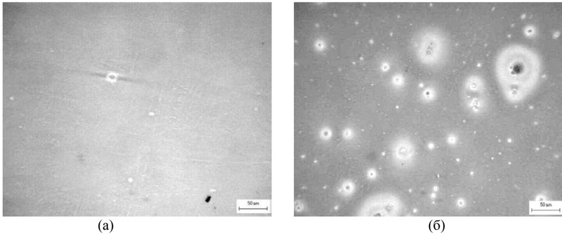
Figure 3: Patch on the glass surface (group  $A_3$ ): a) the glass surface before jet action; b) after jet action.
