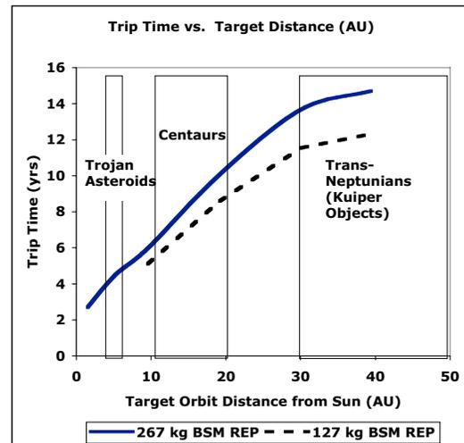
**Figure 5. Trip Times for REP Spacecraft to Co-orbit Primitive Bodies**
