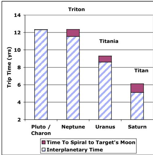
Figure 9. Orbiter Trip Time vs. Object [127 kg BSM]
