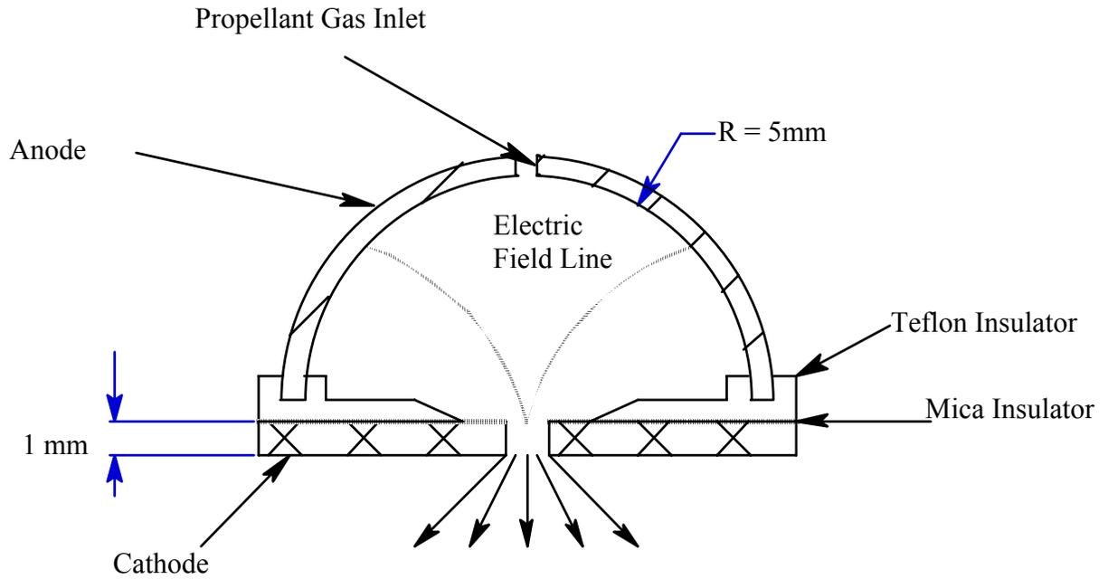
Figure 1: Hollow Cathode Schematic
