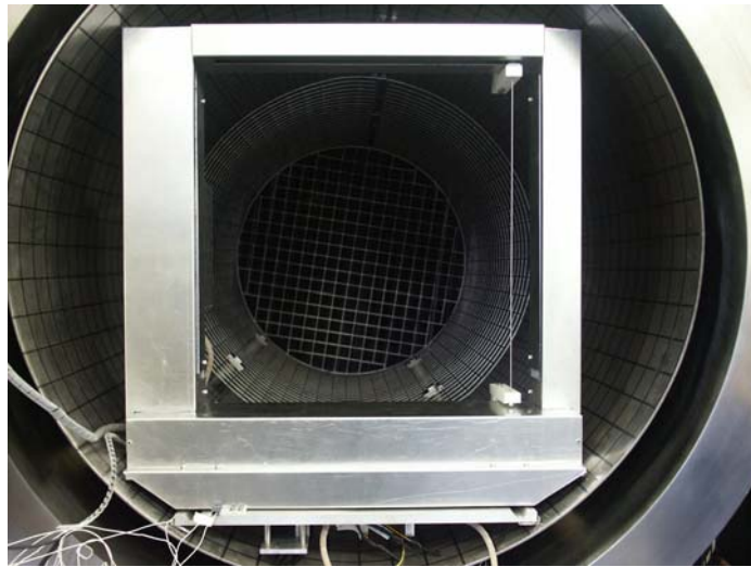
Figure 5 Plasma Diagnostic Facility inside Vacuum Chamber
