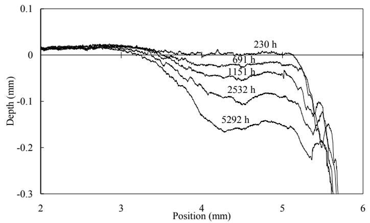
Fig. 5 Eroded depth profiles on the orifice plate downstream surface.
