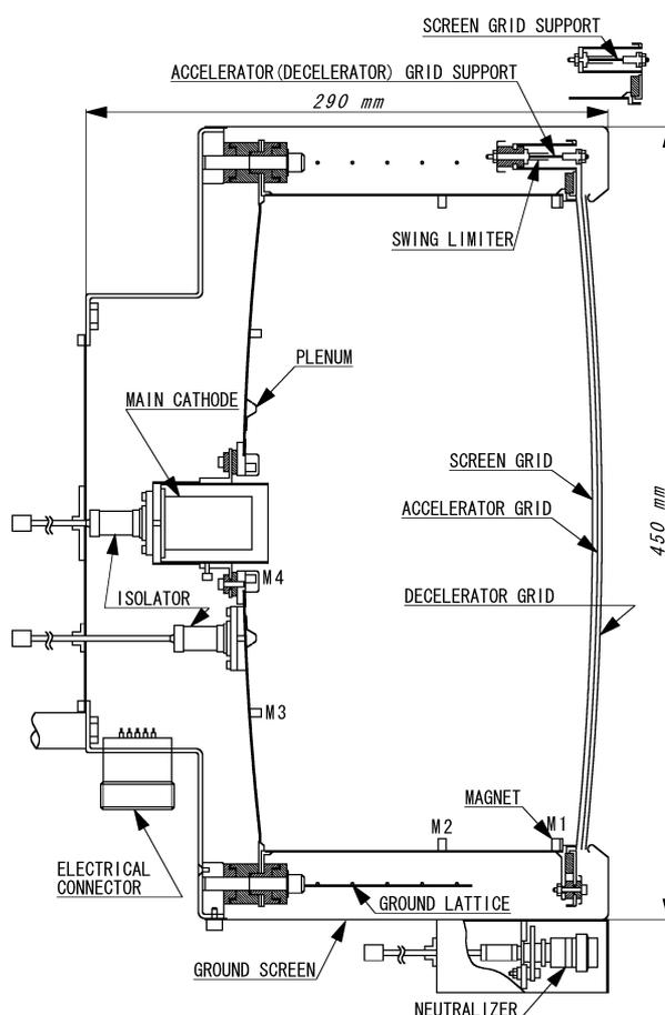
Fig. 1 Sectional view of the BBM-1 thruster.
