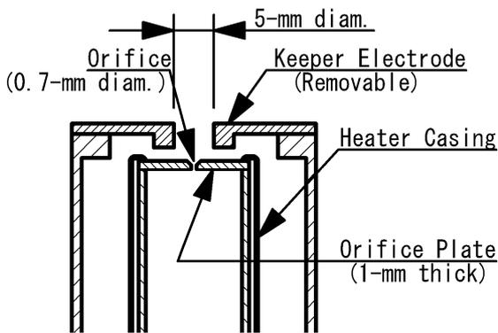
Fig. 4 Cross sectional view of the cathode top.
