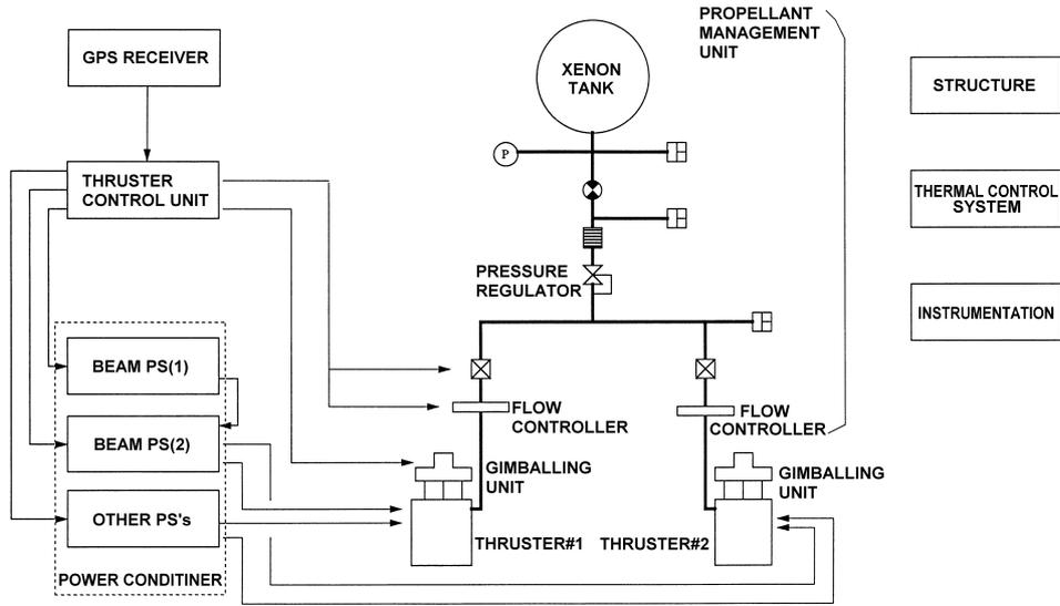
Fig. 6 Functional block diagram of the propulsion system.
