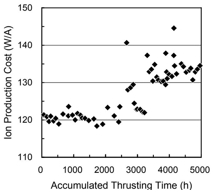
Fig. 3 Variations in the ion production cost in the 5,000-h endurance test.
