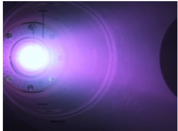
Fig. 1 73.8 cm i.d.(75 cm o.d.)chamber large helicon plasma source run in ISAS by Shinohara and Tanikawa. 3,4
