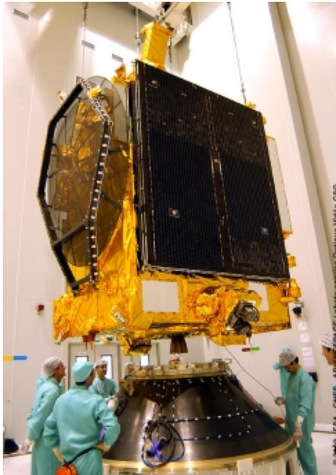
Figure 1 : STENTOR on Ariane 5 Adaptator
