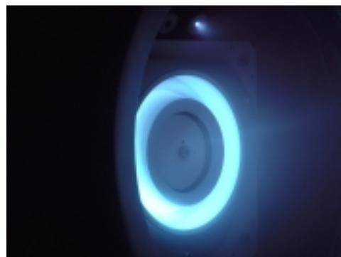
Figure 9 : PPS®X000 technological demonstrator
