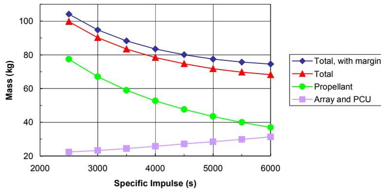
**Figure 3.** Propellant, power system and aggregate masses as functions of SI.
