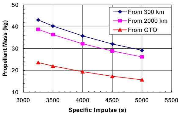
**Figure 1.** Propellant mass as a function of SI for the orbit-raising phase of the mission
