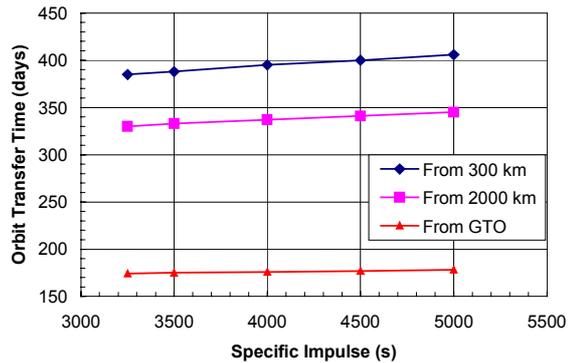
**Figure 2.** Manoeuvre time as a function of SI for the orbit-raising phase of the mission.
