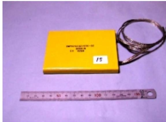
(b) 1.5  $\mu\text{F}$  Plate-Type Capacitor (EM Capacitor)
