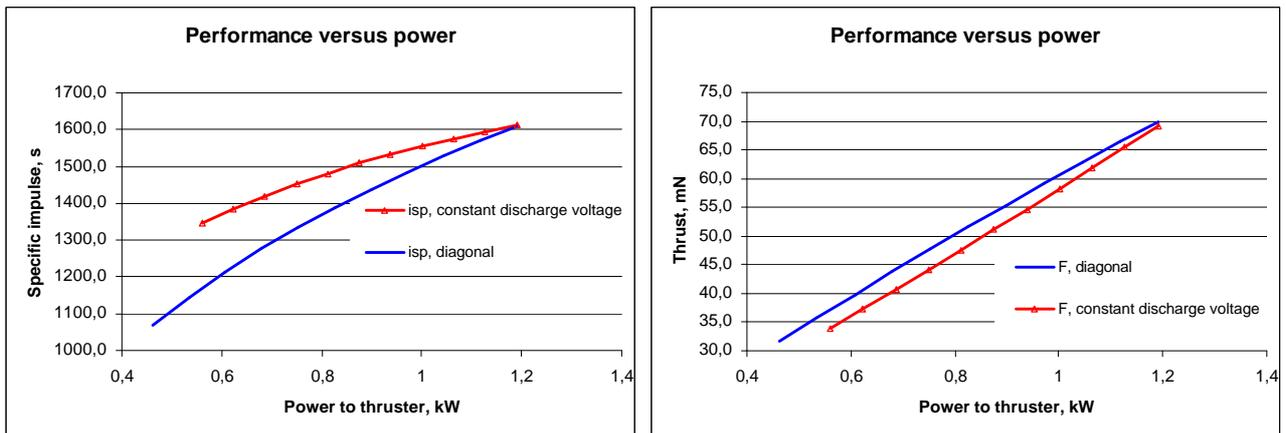
**Figure 15.** Specific impulse and thrust versus power diagonal case and 350 volts case.
