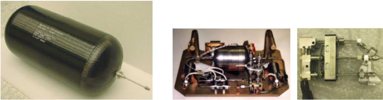
**Figure 2.** Flight model hardware: tank, BPRU and XFC
