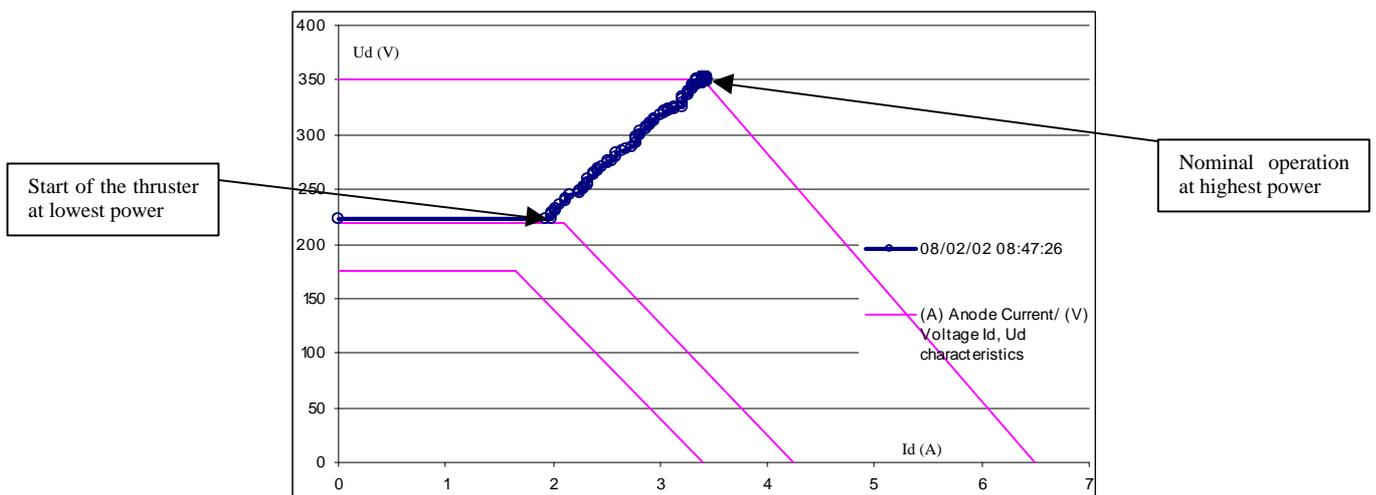
**Figure 18.** Typical PPS<sup>®</sup> 1350-G FM firing at maximum power, starting at low power and following (automatically via the PPU software) the Smart-1 Diagonal
