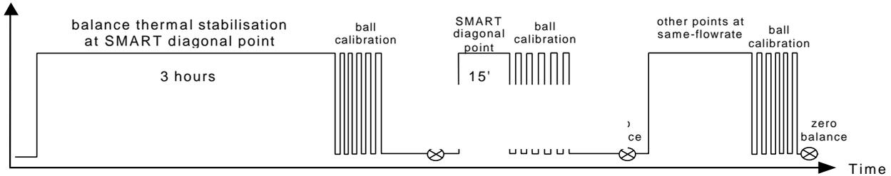
**Figure 11.** Long run test sequence, definition of same flow-rate firing sequence.
