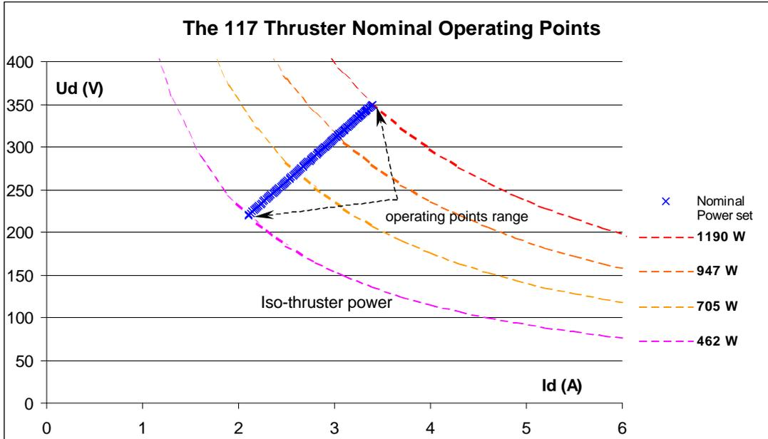
**Figure 7.** The diagonal with the 117 steps of the variable power feature of Smart-1 given by the Nominal Power Set parameter. The EPS Power at thruster level is of course  $U_d \cdot I_d$ , some iso-Power hyperbola are shown.
