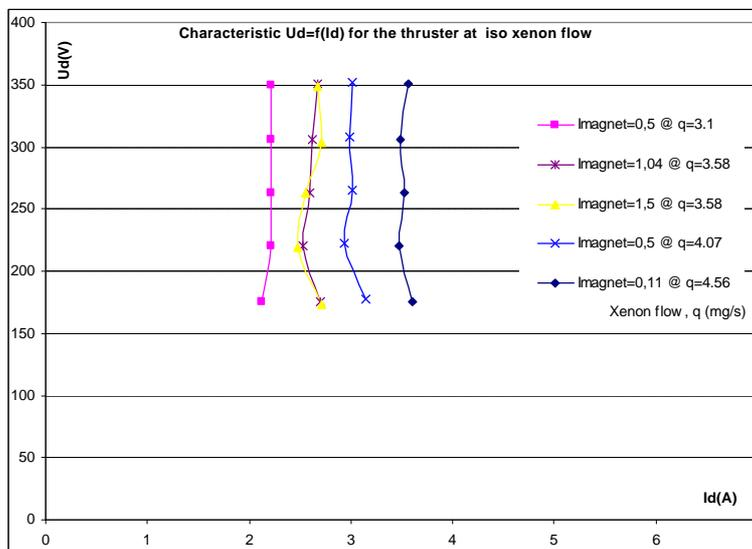
**Figure 8.** Thruster characteristics, power at thruster level is of course  $I_d \cdot U_d$
