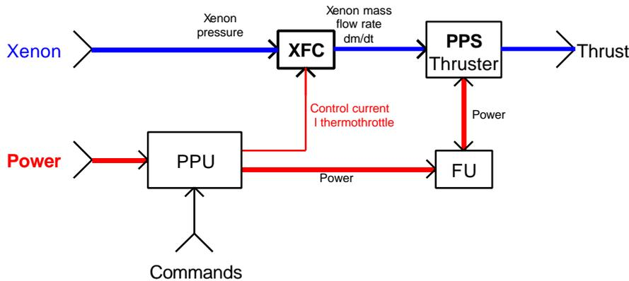
**Figure 5.** Xenon flow regulation loop
