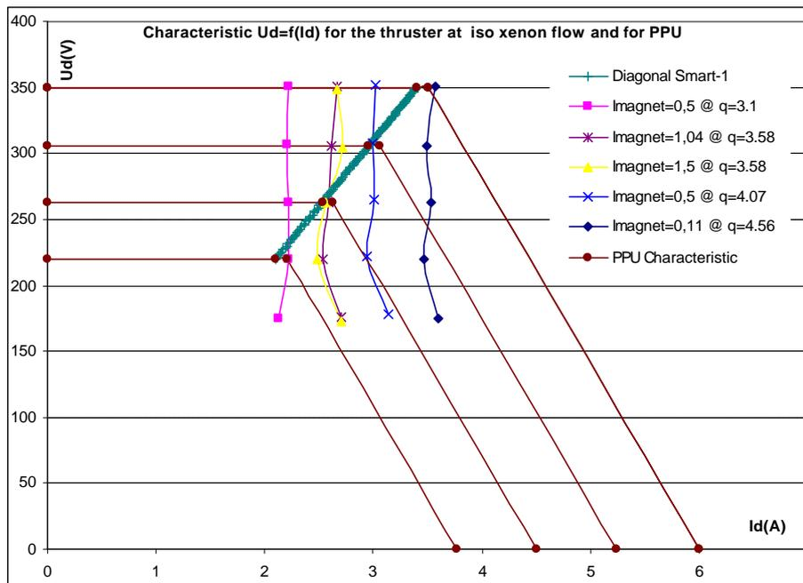
Figure 10. The whole characteristic of PPU/TSU, thruster with the Smart-1 diagonal
