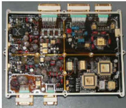
**Figure 17.** PRE Card FM after functional tests at Atermes (with savers connectors)
