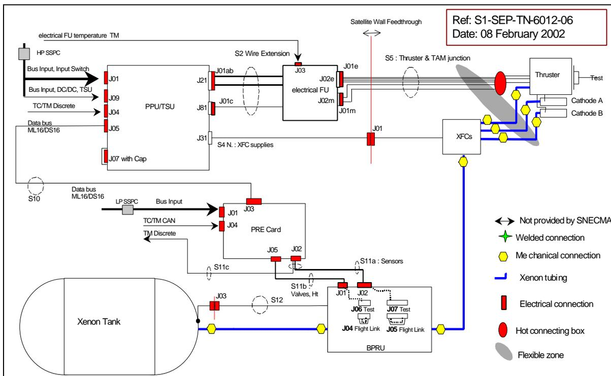
**Figure 1.** EPS functional diagram: the xenon system feed the thruster cathodes and anode
