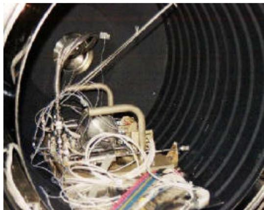
**Figure 16.** BPRU thermal vacuum functional tests with real xenon gas, at Madrid INTA facility
