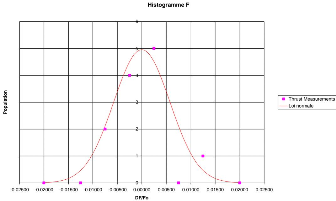
**Figure 14.** Show of the dispersion on 4 sets of 3 identical measurements performed on the first diagonal, Standard deviation  $\sigma$  expressed as  $\Delta F / F_o$  is 0.00575. The overall thrust accuracy measurement at  $3\sigma$  is  $\pm 1.7\%$  .
