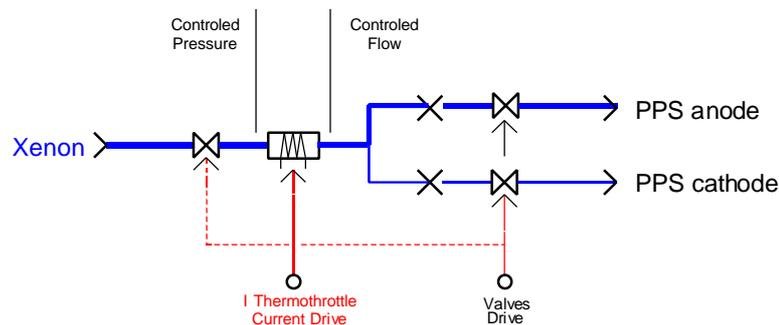
**Figure 6.** Xenon flow Controller functional diagram
