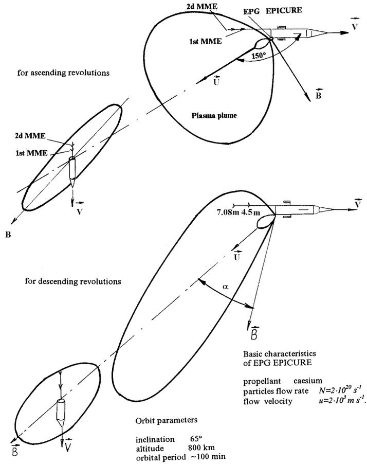
Figure 4 Shape of plasma plume in EPICURE experiment
