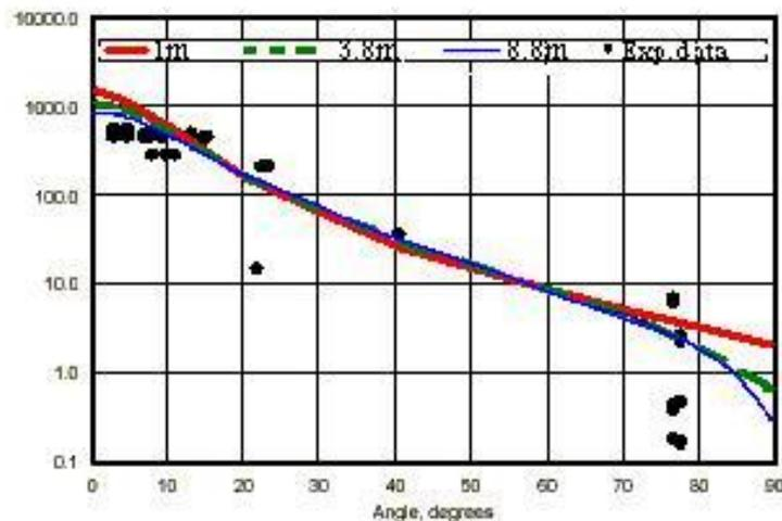
**Figure 1 Comparison of *Express* experimental data and SSM-distribution of axial current density,  $j_x$ , for different distances .**
