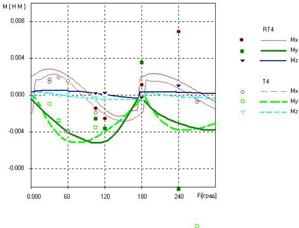
**Figure 3 Comparison calculated torque with Express data for T4, RT4 [14]**
