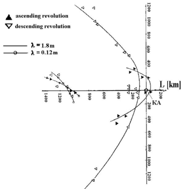
Figure 5 Shape of the radio shadow on Earth surface.
