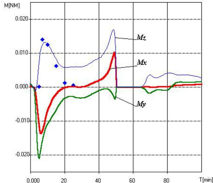
**Figure 9 Flight data and theoretical dependencies of change of torque components during one orbit period of Meteor SC.**
