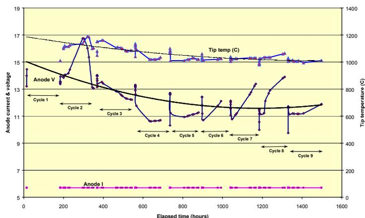
**Figure 10 Evolution of operating parameters (contaminated cycles only)**
