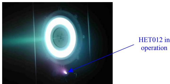
**Figure 13 First firing of HET012 (photograph courtesy of Astrium Ltd)**
