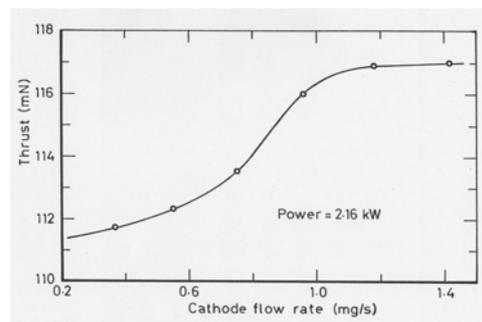
**Figure 5 Performance of thruster using cathode prototype 1**
