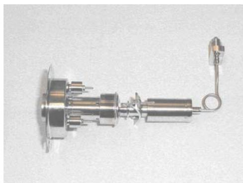
Figure 1 3.6A Discharge Cathode for Artemis
