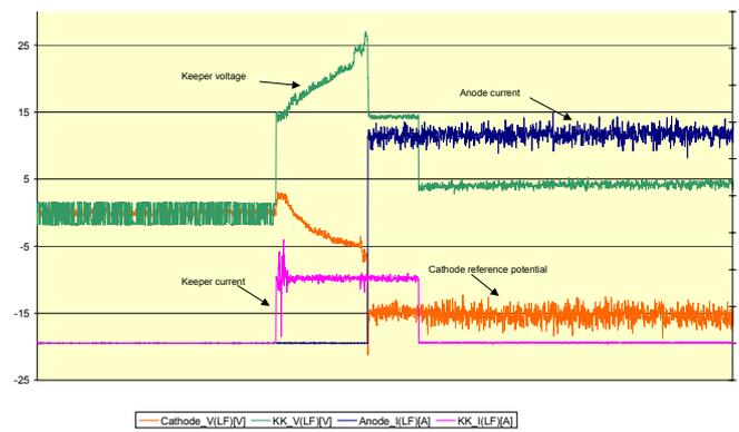
**Figure 15 HET010 Characterisation Test (4<sup>th</sup> July 2002)**
