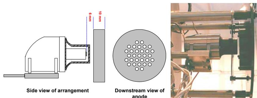
**Figure 9 Cathode in Diode Mode**
