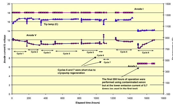
**Figure 12 Evolution of anode and temperature operating parameters**
