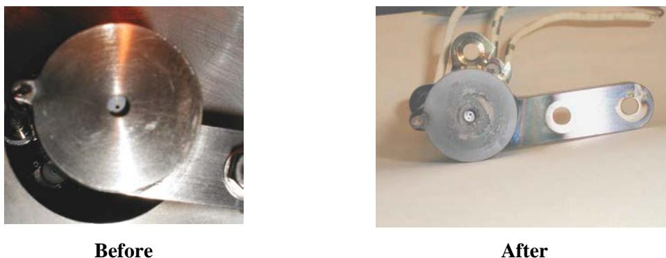
**Figure 2 Downstream view of neutraliser before and after 1000 hours operation in poor vacuum**
