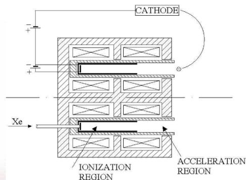
**Fig. 5 - Low Energy Electron Accelerator for layer-by-layer composite curing, left; laboratory prototype of small tank prior to be submitted to electron irradiation for polymerization, middle; conceptual scheme of the proposed double stage Hall thruster, right.**
