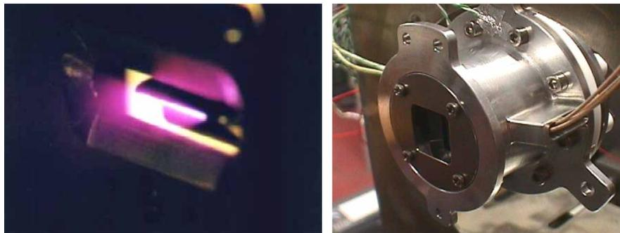
**Fig. 7 - Rb-fed FEEP thruster plume, left; 100  $\mu\text{N}$  thruster module, right.**
