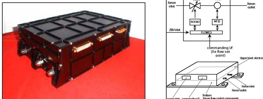
**Fig. 4 -GFCU EM developed for the RMT thruster, left; proposed configuration for the innovative GFCU, right.**
