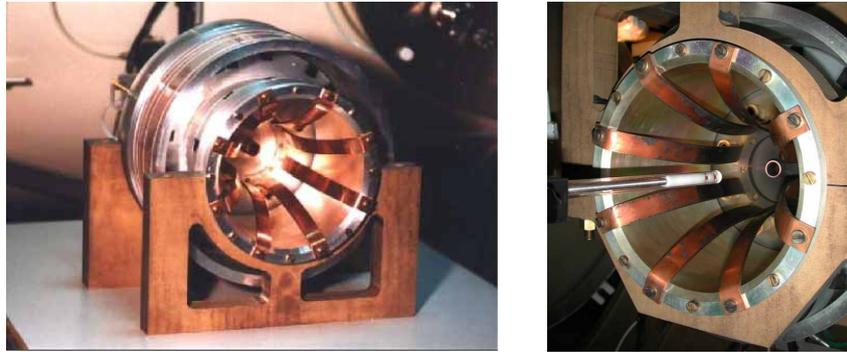
**Fig. 10 - Centospazio's HPT prototype: on the bench, left; with a magnetic probe assembly, right.**
