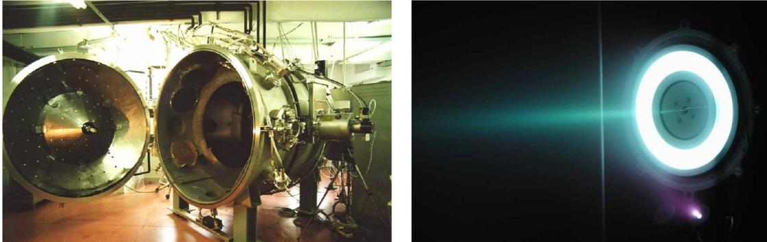
**Fig. 14 - Alta's IV4 test facility: 2 m diameter, 3.2 m long, with an additional 1 m diameter, 1 m long lock chamber; a 1 m diameter gate valve connects the two. At right, Astrium's ROS-2000 HET fired in Alta's IV-4 facility.**
