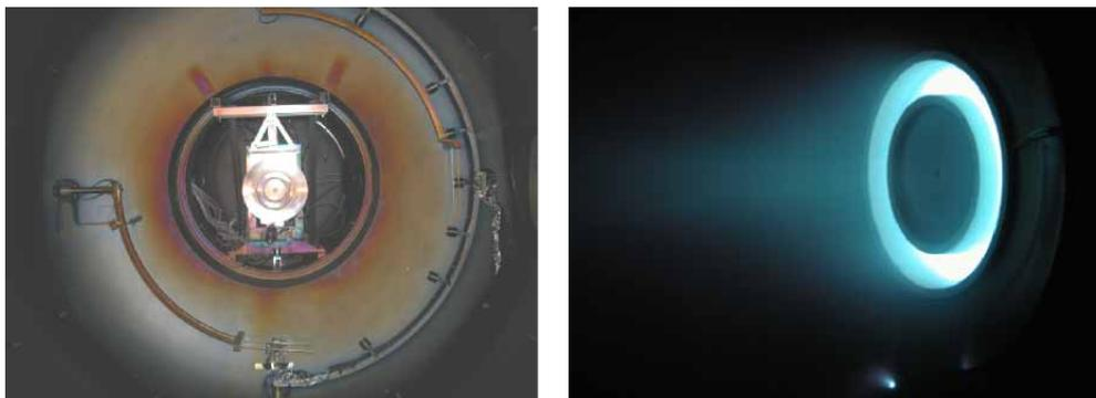
**Fig. 13 - Alta's 5 kW Hall thruster in facility IV4.**
