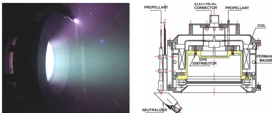
**Fig. 1 - RMT Ion Thruster: under test at LABEN/Proel, left; cross section drawing, right.**
