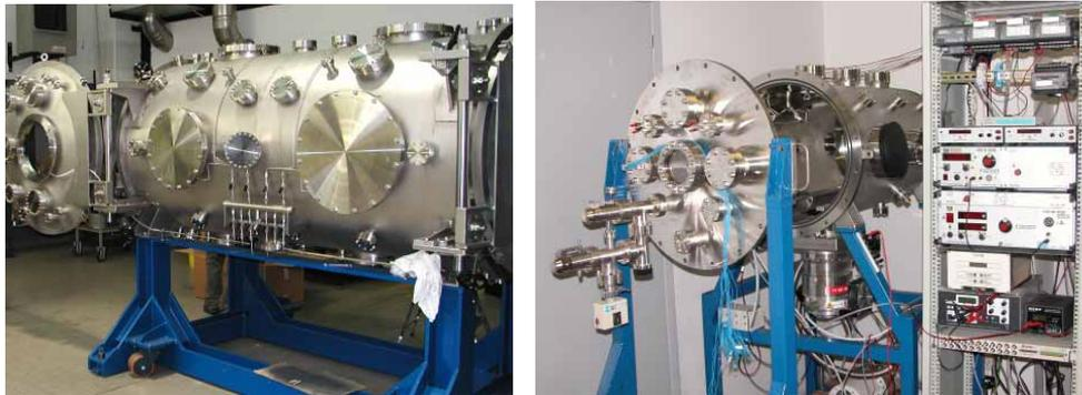
**Fig. 9 - The FEEP lifetime and qualification test facility, left; one of three identical support test chambers, right.**
