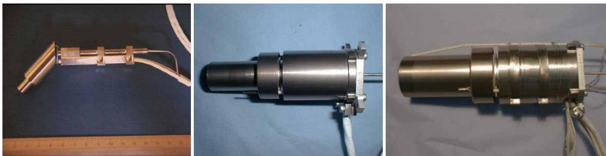
**Fig. 2 -Neutralizer for the RIT 10 thruster on ARTEMIS, left; cathode for the PPS 1350 Plasma Thruster, middle; cathode for the PPS X000 (usable also for the RIT-XT on Alphas), right.**
