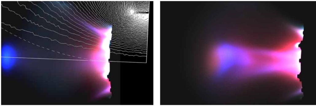
**Fig. 12 - Picture of the HPT plume with calculated superimposed applied magnetic field, left; a plasma “clot” after expulsion, right.**
