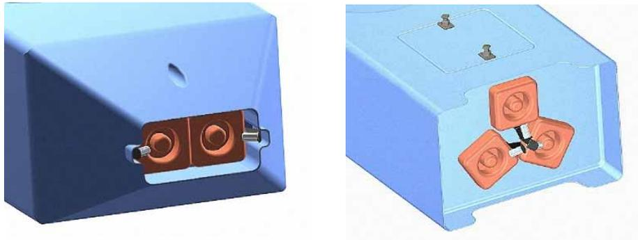
**Fig. 5 - Hall thruster locations: ram side, left; wake side, right.**
