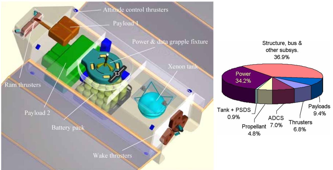
**Fig. 3 - Subsystem configuration and mass breakdown**
