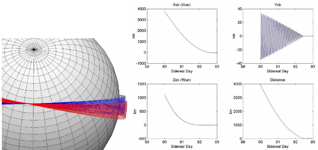
**Fig. 7 - Orbit planes shift reduction: ISS orbits in blue, MOV orbits in red (left). Time history of the relative distance during the rendezvous phase, right.**
