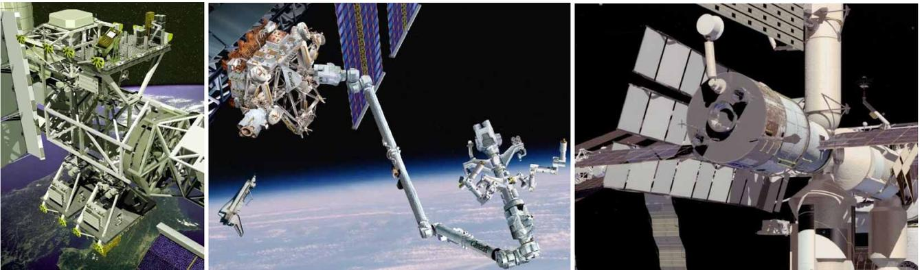
**Fig. 1: Express Pallet platforms on the Main Truss, left; Remote Manipulation System “Canadarm” and Special Purpose Dexterous Manipulator, middle; Russian module “Zvezda”, right.**
