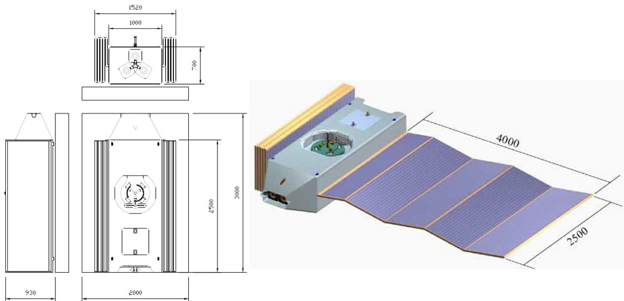
**Fig. 2 - MOV dimensions (in mm) mounted on the Express Pallet platform, left; MOV solar array dimensions (in mm) with port array deployed, starboard array folded (right)**
