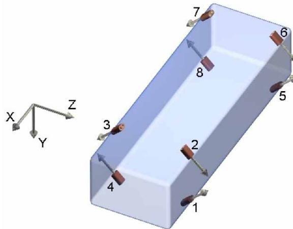
**Fig. 4 - Attitude control thruster locations and thrust vector orientations.**
