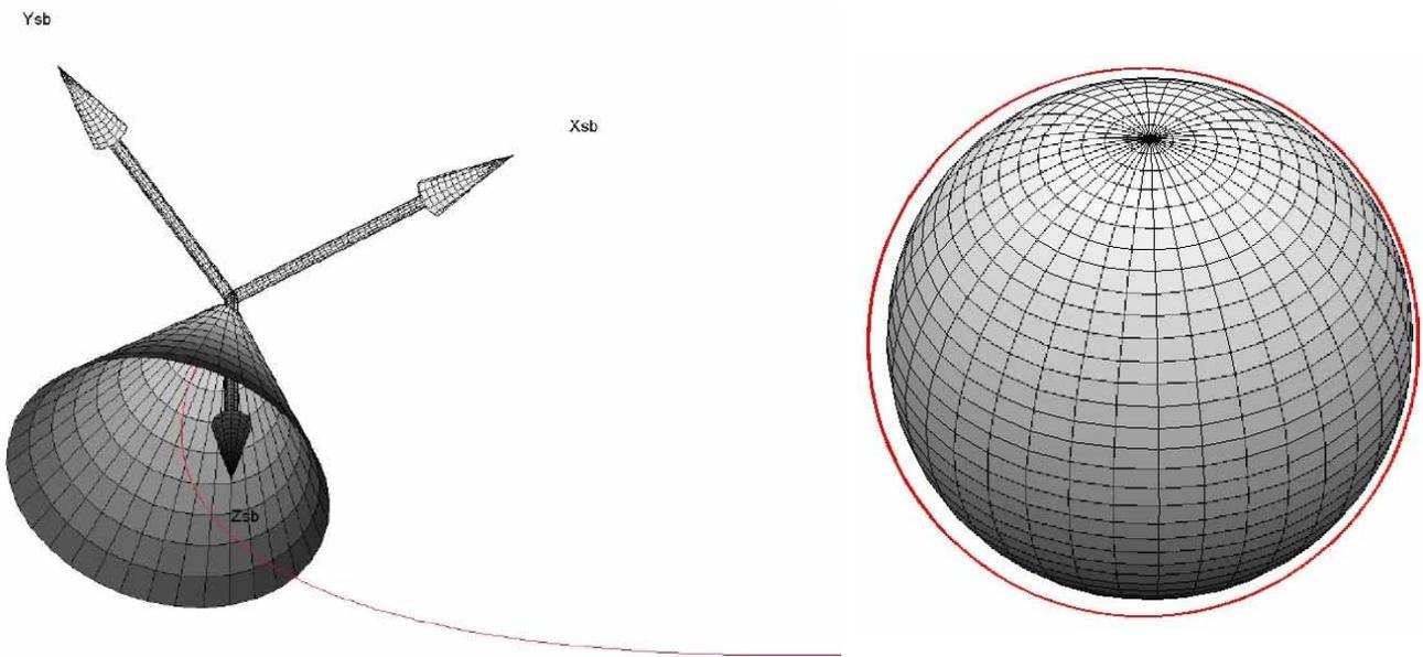
**Fig. 6 - Departure from the ISS through the departure cone, left; operational orbit (drawing to scale), right.**
