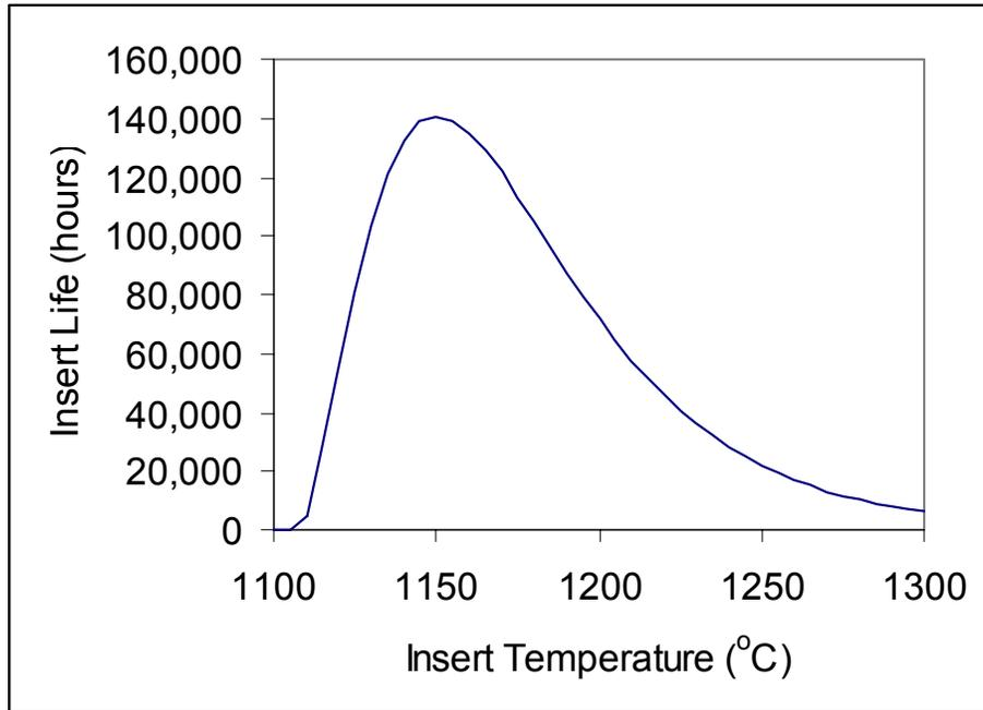
Figure 3. Expected insert life for the space station cathode as a function of insert temperature
