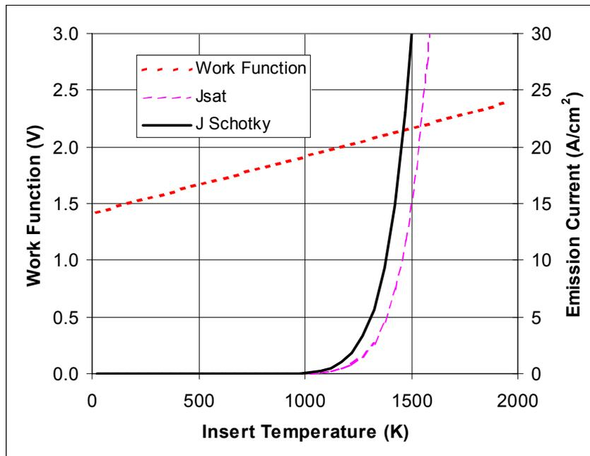
Figure 2. Work function and saturation emission currents with and without the Schotky electric field enhancement term.
