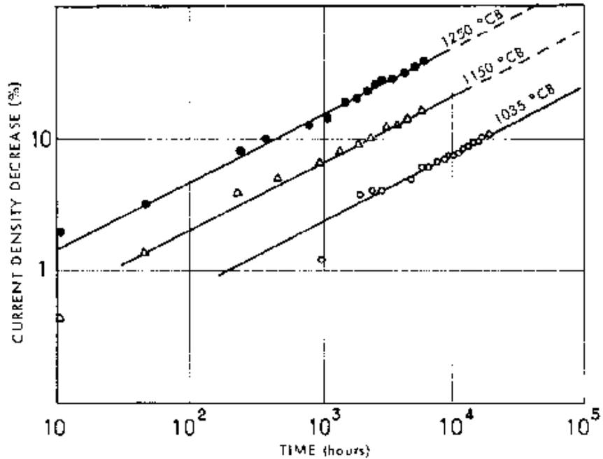
Figure 1. Decrease in saturation emission current with time for different cathode temperatures. Figure from Palluel and Shroff [3].
