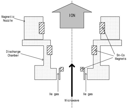
**Fig. 1 Schematic of the microwave engine's cross section**
