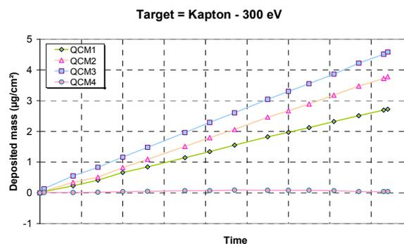
Fig. 7 – QCM measurements during Kapton-300 eV contamination test
