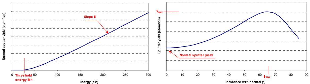
Fig. 2 – Energy and incidence dependence of sputter yields
