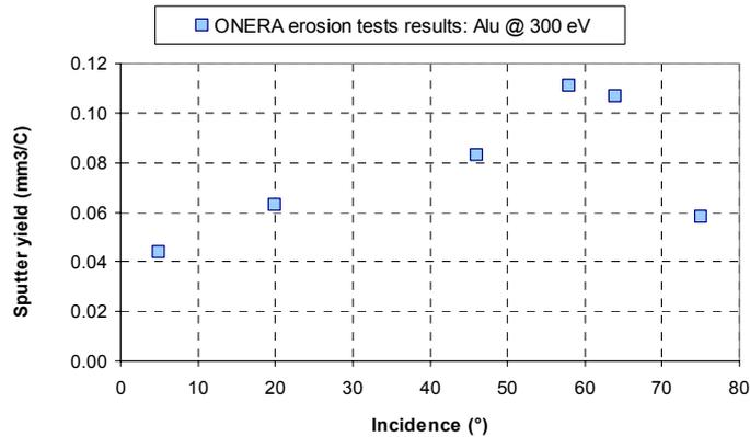
Fig. 5 – Example of aluminium sputter yields at 300 eV\*
