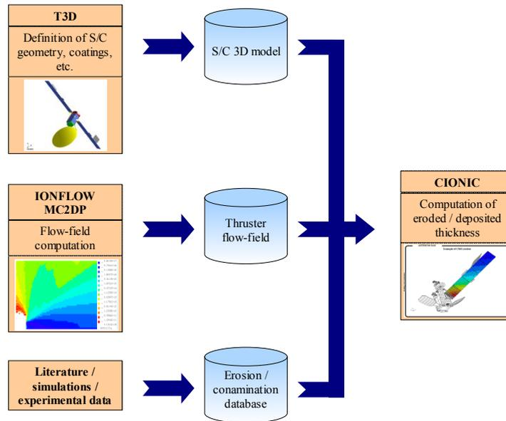
Fig. 1 – Software architecture of CIONIC
