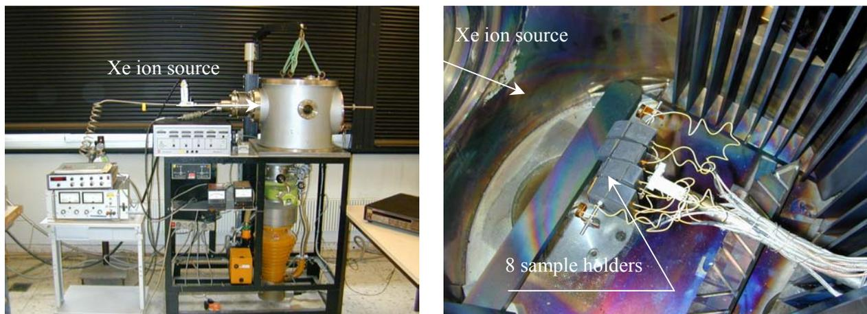
Fig. 4 – ONERA erosion test set-up
