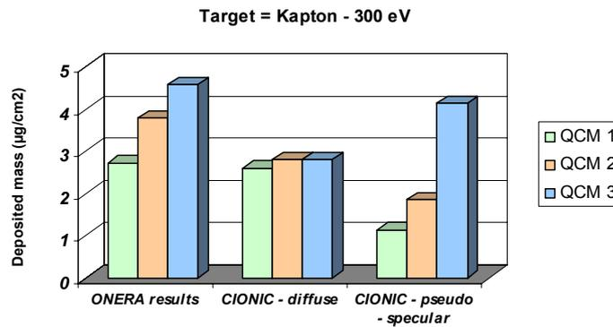
**Fig. 10 – Comparison between ONERA QCM measurements, and Astrium predictions with both re-emission laws**
