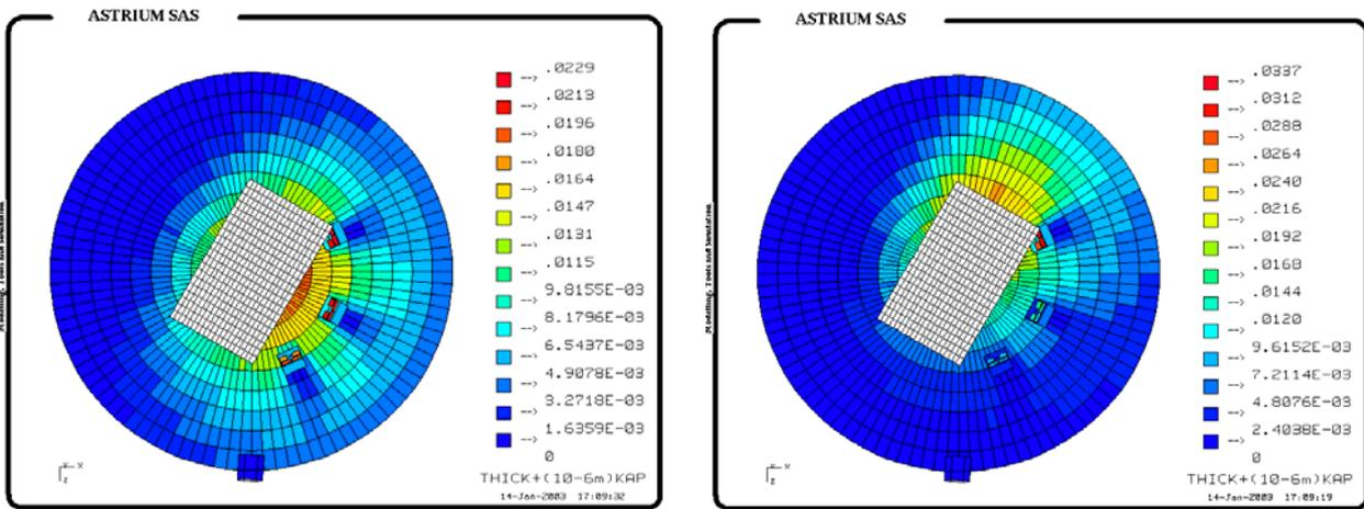
**Fig. 9 – Example of predicted contamination in the case of Kapton 300 eV test:**
