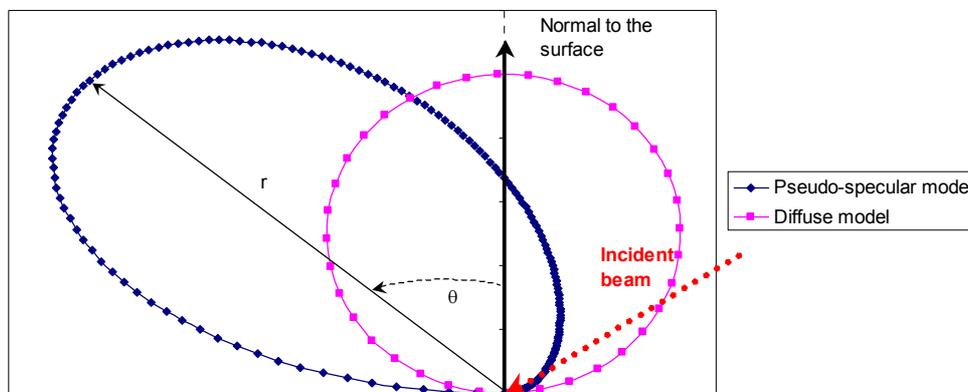
Fig. 3 – Diffuse and pseudo-specular re-emission lobes
