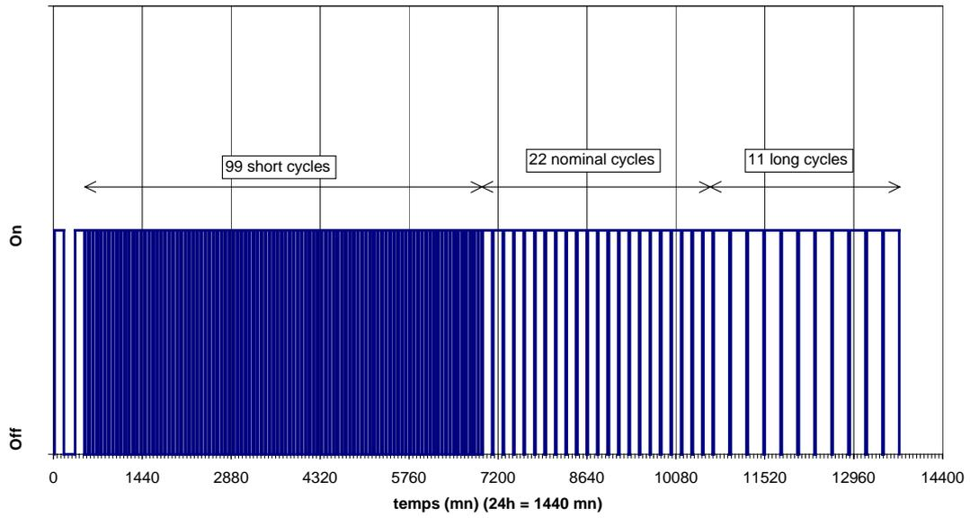
Fig. 7 : typical On/Off sequence during life test
