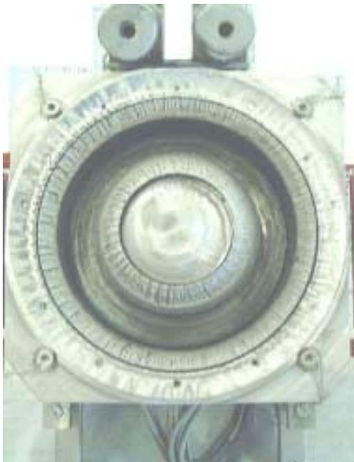
Fig. 4 : PPS® 1350 MI thruster after lifetimes
