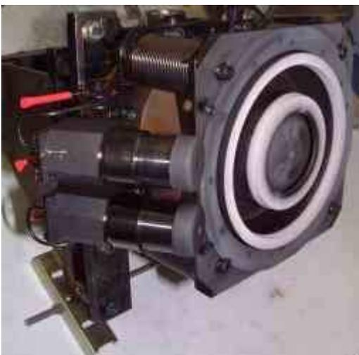
Fig 3 : PPS® 1350-G MQ on its tooling for acceptance thermal cycling
