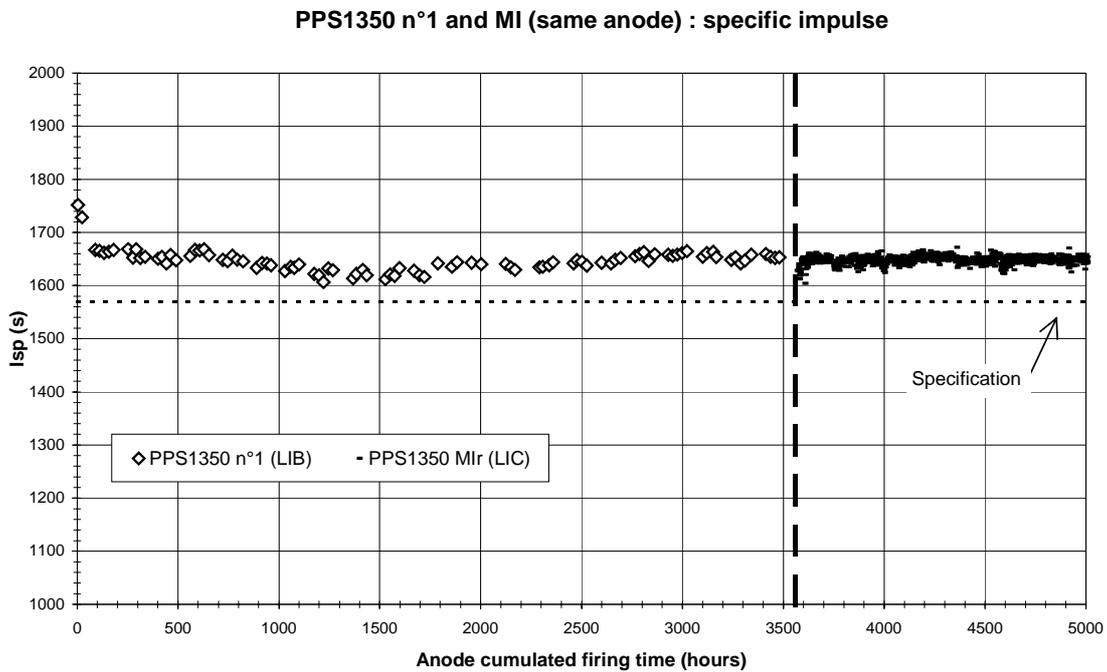
Fig. 6 : PPS 1350-G type Chamber and anode : Specific Impulse
