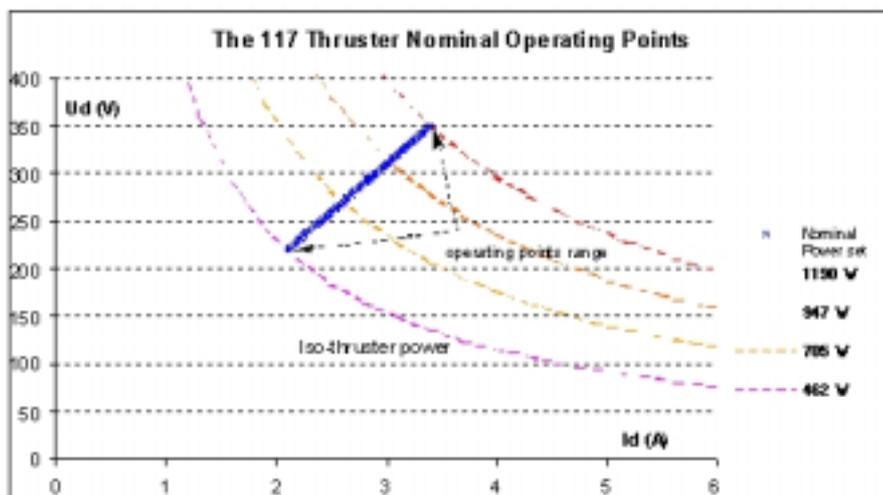
Fig.8 : The diagonal with the 117 steps of the variable power feature of Smart-1 with some iso-Power lines
