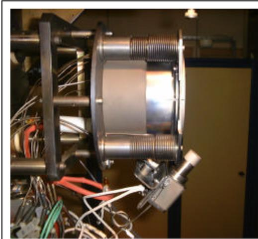
**Fig.8: Ncca 5000 HCA assembled together the SPT 100 ML thruster at CNRS labs**
