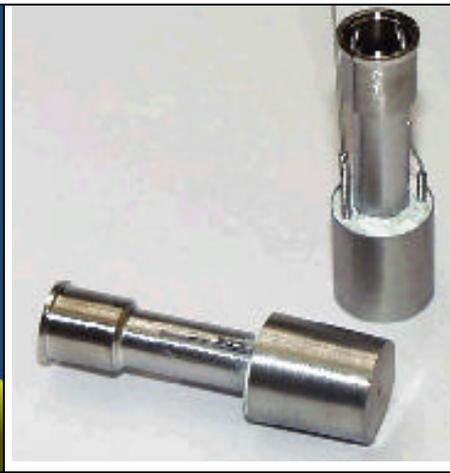
**Fig. 16: HP HCA Emitter Prototypes**
