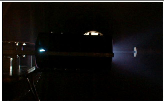
**Fig. 20: HP HCA in operation within the vacuum chamber**
