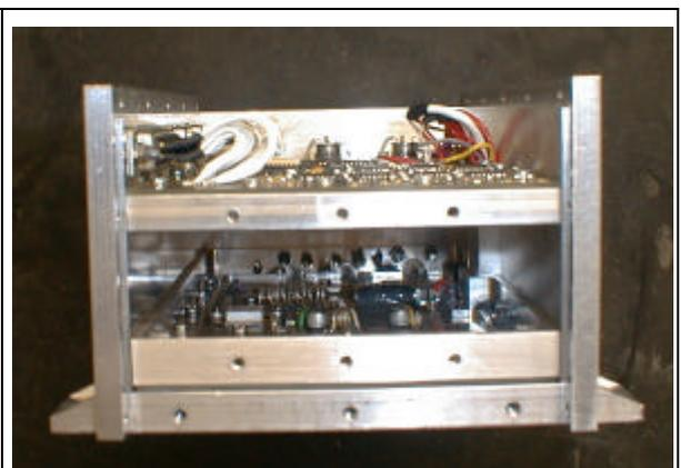
**Fig. 10: RFGU housing box opened to show the accommodation of the electrical parts**
