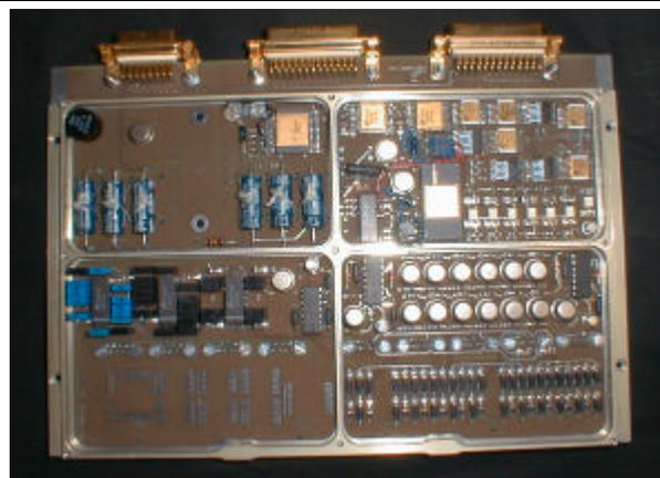
**Fig. 8: GFCU PCB dedicated the command/ control of the GFCU operation**
