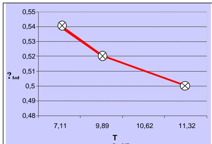
**Fig. 13: Plot of the thruster efficiency versus thrust level**
