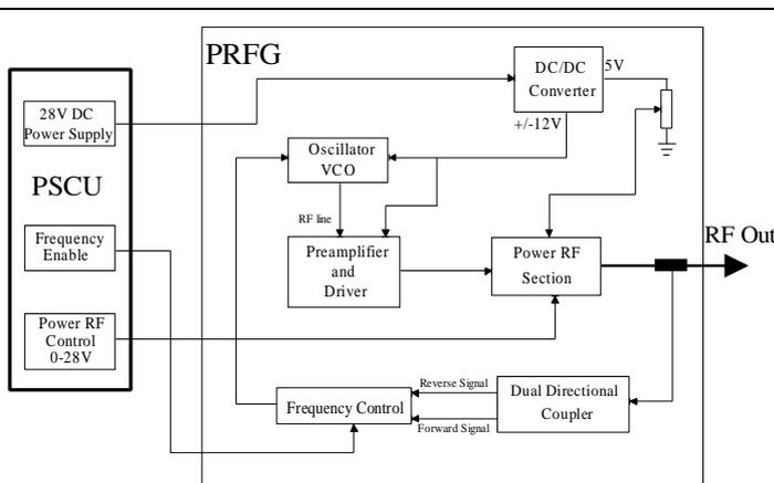
**Fig. 9: RFGU functional Block Diagram**
