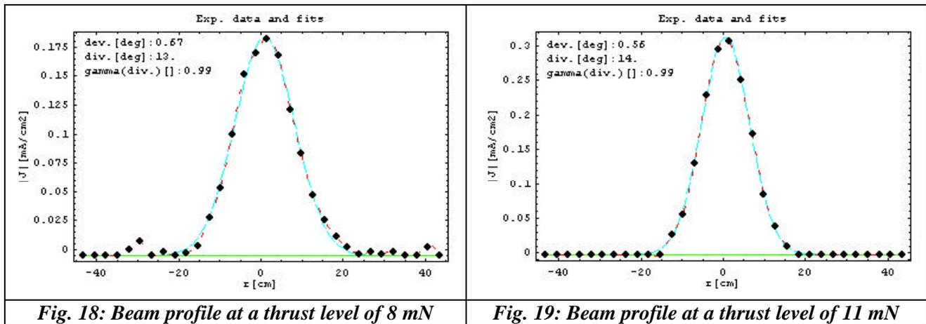
**Fig. 18: Beam profile at a thrust level of 8 mN**
