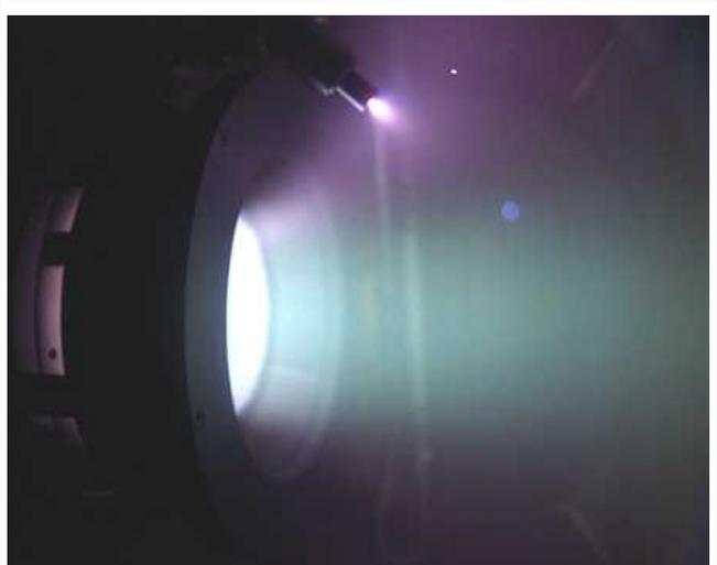
**Fig. 12: RMT under functional test**
