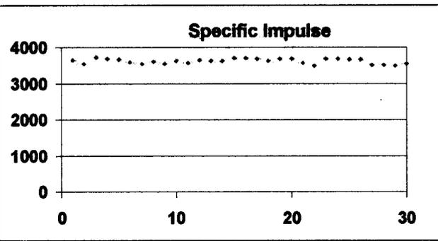
**Fig. 15: Evolution of the Specific Impulse versus time**
