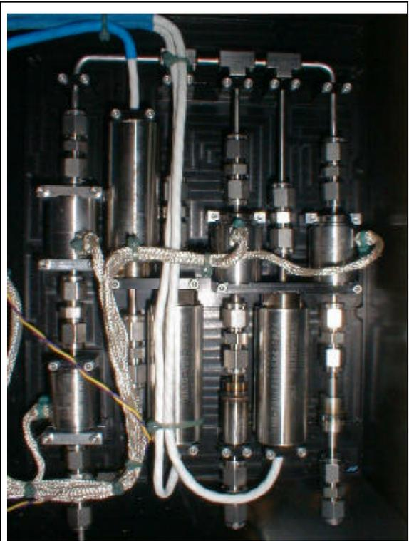
**Fig. 6: Photo of the GFCU Flow Line Section**
