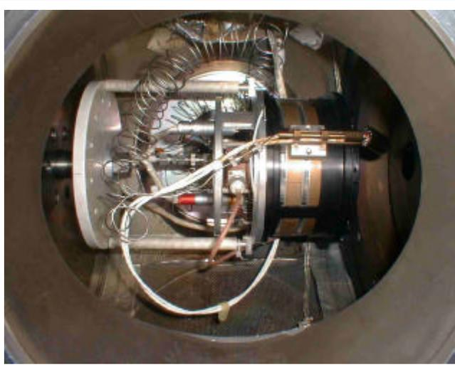
**Fig. 11: RMT integrated into the vacuum chamber**
