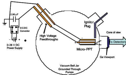
Figure 8: Experimental layout used for thruster IR data.
