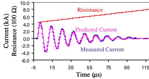
Figure 9: Comparison of measured and calculated current with linearly varying resistance.
