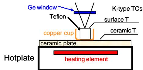
Figure 6: Calibration procedure in-tank layout.
