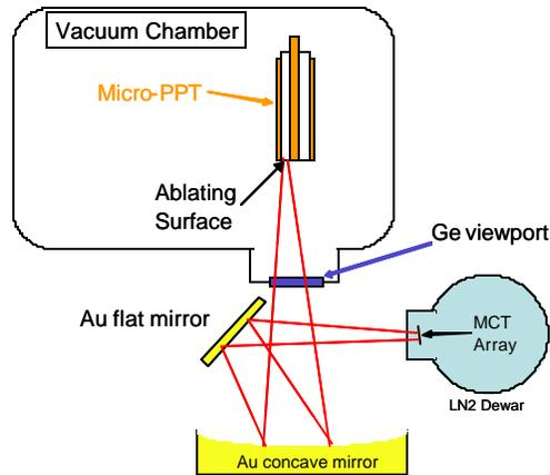
Figure 5: IR detector experimental layout.
