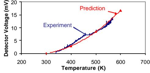
Figure 7: Measured and predicted Teflon response.
