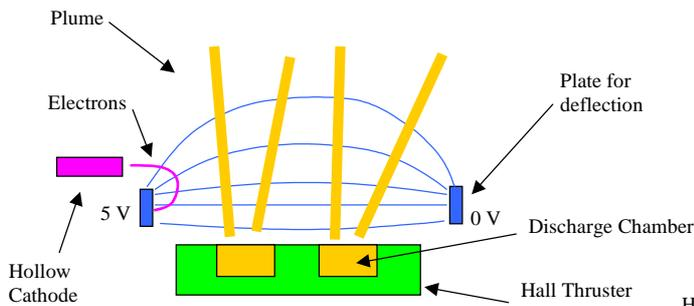
Fig. 6 – Electrons going toward the deflecting plates
