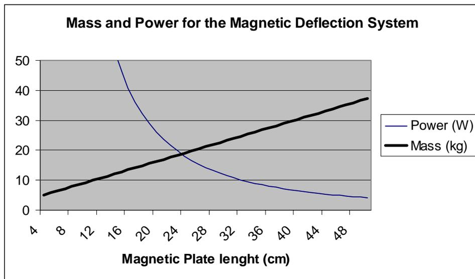
Fig. 10 – Needed mass and power for the magnetic deflection of the Hall thruster plume
