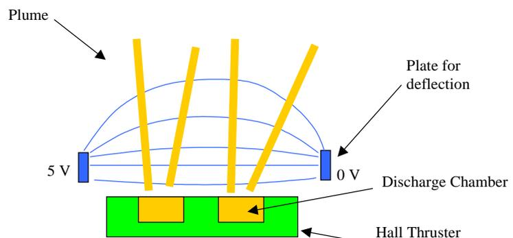
Fig. 5 – Electric field non-uniformity
