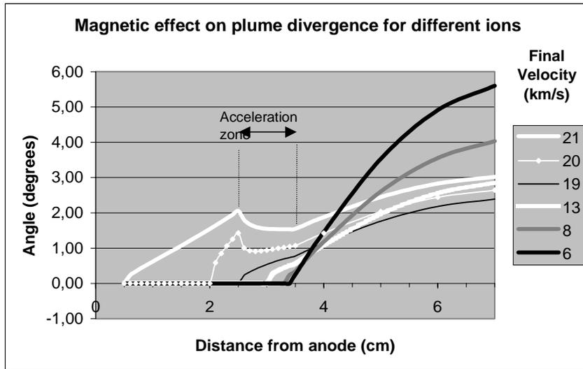
Fig. 4 – Magnetic effect on plume divergence for ions created at different distances from anode.
