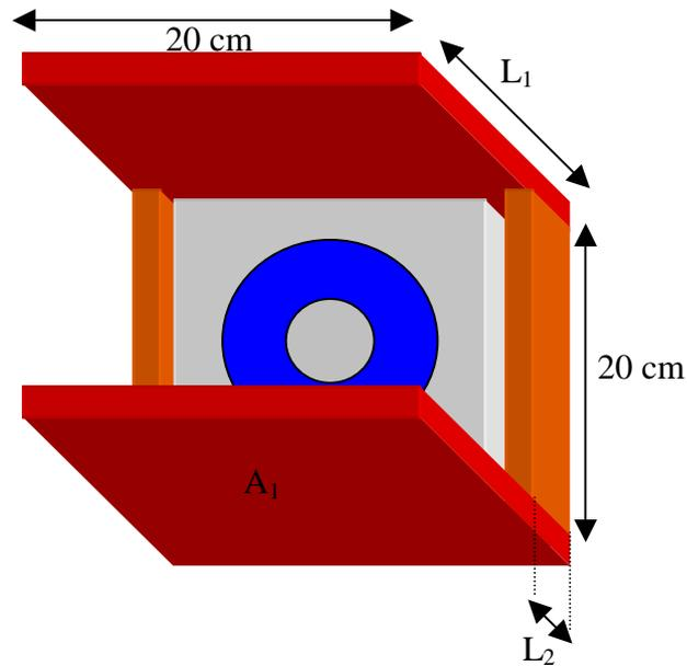
Fig. 9 – Magnetic system for plume deflection
