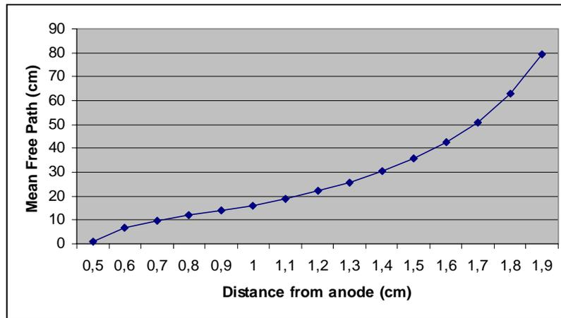
Fig. 1 – Mean free path versus anode distance for elastic collisions
