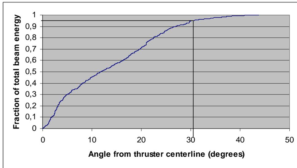
Fig. 13– Fraction of total beam energy vs angle for a PIC code with few particles.
