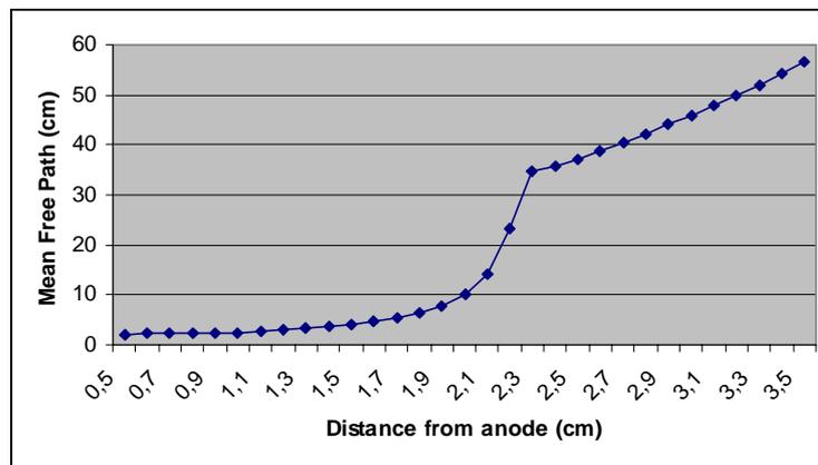
Fig. 3 – Mean free path for charge exchange collision
