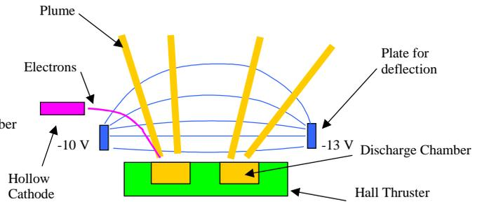
Fig. 7 - Divergence of the plume created by the deflecting plates
