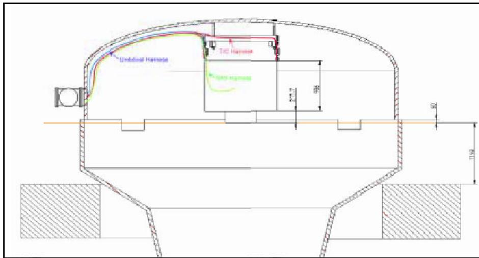
**Figure 3: Spacecraft Configuration and Harness Routing in HBF-3**
