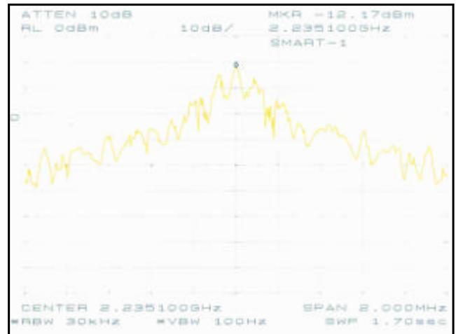
Figure 10: Downlink spectrum during EP full power
