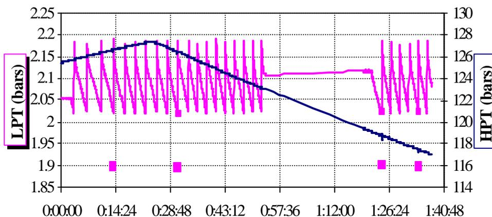
Figure 17: Tank and Plenum Pressures during E2E
