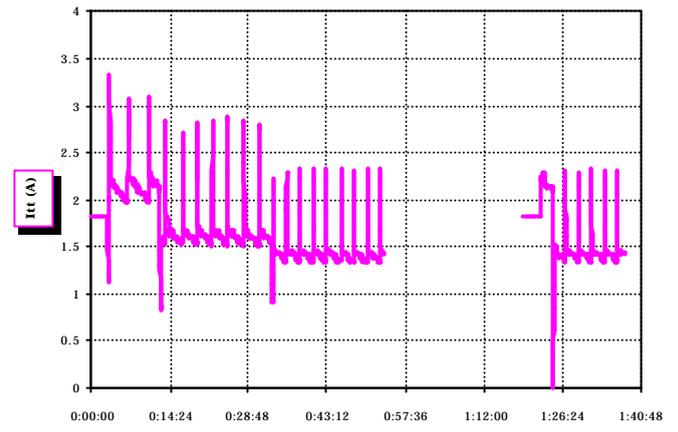
Figure 16: Thermothrottle Current during E2E
