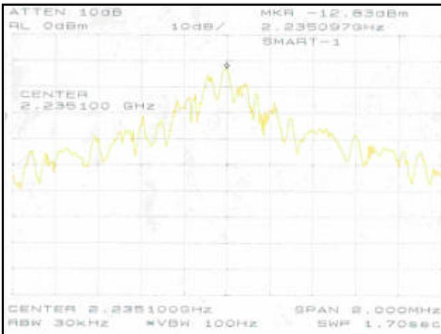
Figure 9: Downlink spectrum during venting phase
