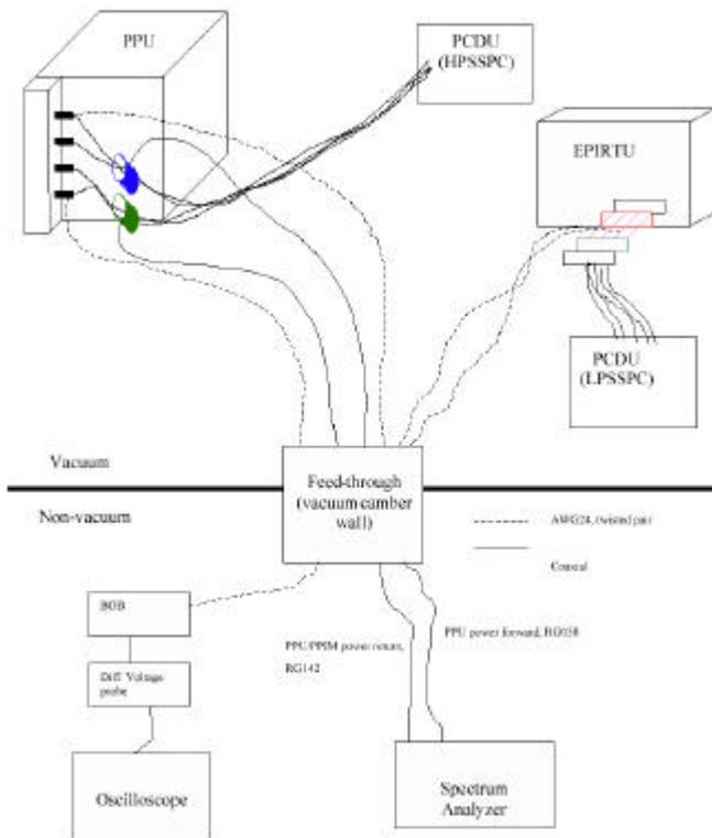
Figure 4: Conducted EMC Test Setup for EP
