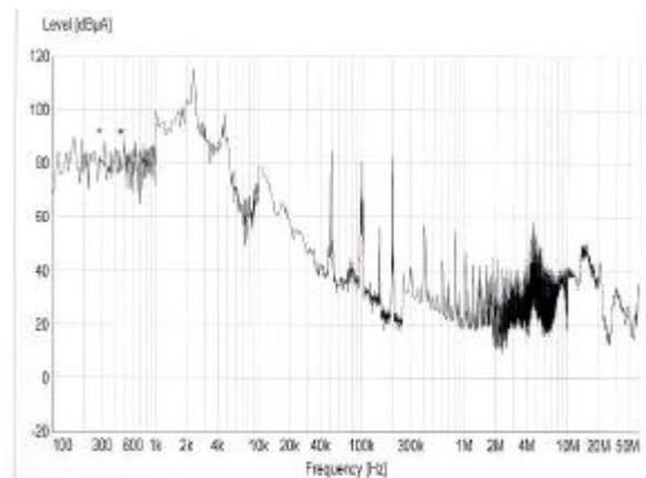
Figure 7: PPU, 100Hz-50MHz, 1200W system EMC
