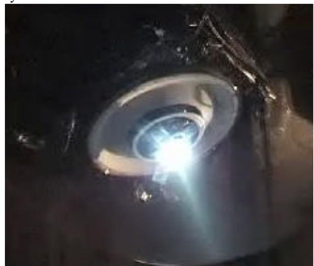
After the firing tests, the spacecraft was left under vacuum conditions until the thruster mechanical interface had recovered its initial temperature from before the test. The HBF-3 vacuum was then broken with nitrogen flushing in order to slowly recover ambient pressure conditions. After chamber opening, all the contamination samples were inspected as well as all the spacecraft optical properties.
