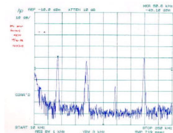
Figure 6: PPU, 10-250kHz, 1200 W discharge
