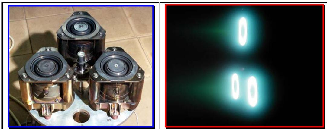
Fig. 3. Three Cluster of three D-55 assembly.
