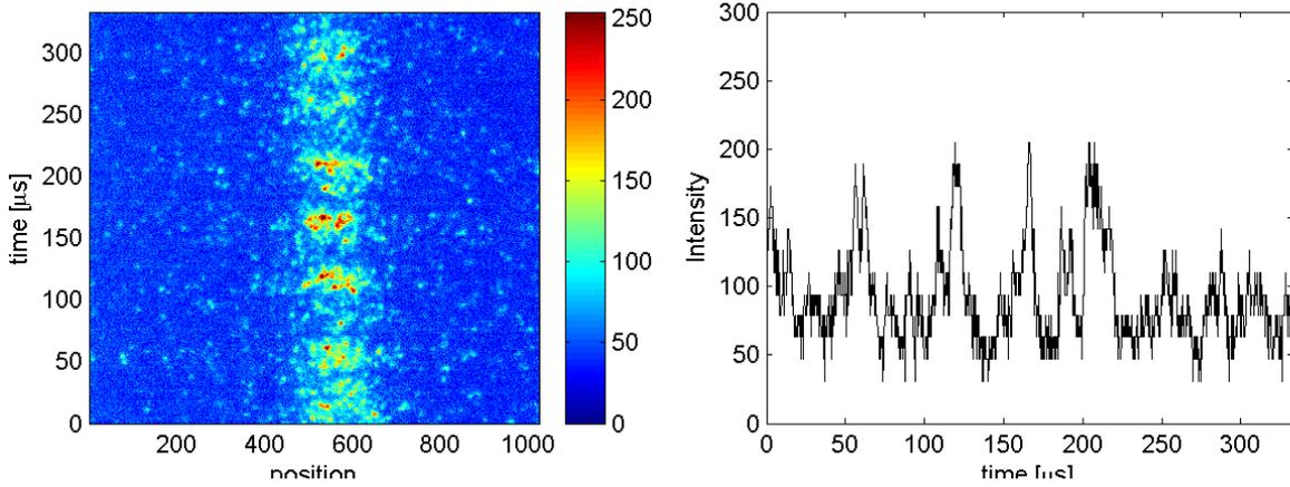
Fig. 8. Streak images of plasma emission with image of streak camera slit aligned perpendicular to the drift direction as seen in Fig. 3. Left: full image ( $330 \mu\text{s} \times 2 \text{ cm}$ ). Right: Single-pixel stripe through the position corresponding to about the channel centerline.
