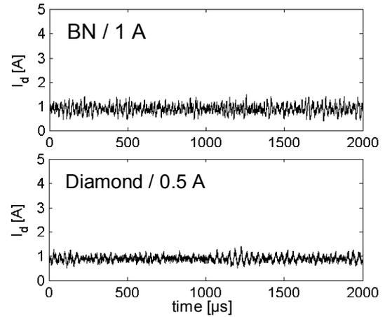
Fig. 4. Oscillogram of the discharge current for boron nitride walls (1 A magnet current) and diamond walls (0.5 A magnet current).
