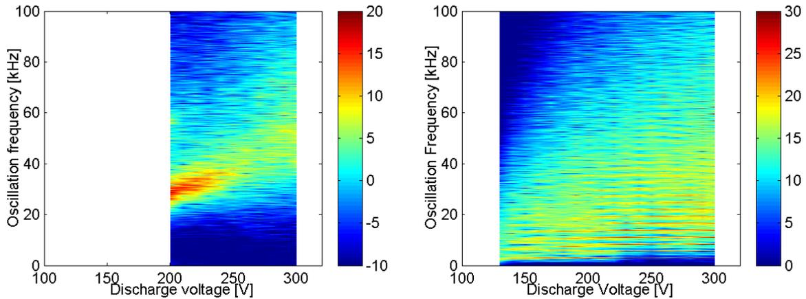
Fig. 7. Spectral maps for the discharge conditions as those cases shown in Fig. 6. Left: Operation with boron nitride walls. Right: Operation with diamond walls.
