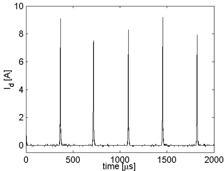
Fig. 5. Oscillogram for the case of diamond walls, with the discharge in the “pulsed” mode (1A magnet current).
