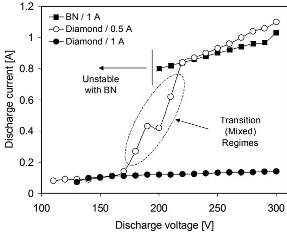
Fig.3. A comparison of the I-V discharge characteristics of the linear thruster with either boron nitride or diamond walls.
