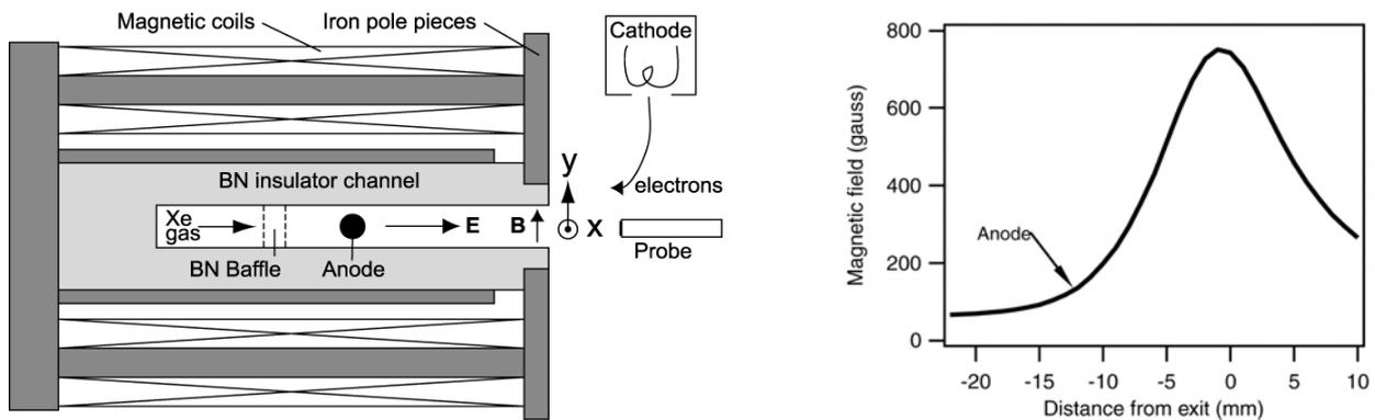
Fig. 1. Left: Linear Hall thruster design details. Right: Magnetic field profile.
