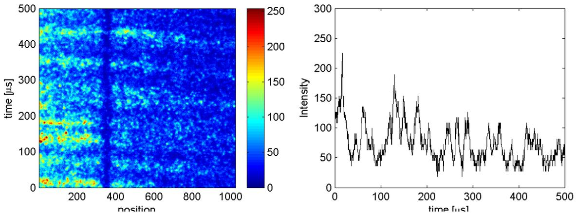
Fig. 9. Streak images of plasma emission with image of the streak camera slit aligned along the drift direction as seen in Fig. 3. Left: full image ( $500 \mu\text{s} \times 2 \text{ cm}$ ). Right: Single-pixel stripe through the position corresponding to the 200<sup>th</sup> pixel column (favoring the side of the thruster towards  $\mathbf{E} \times \mathbf{B}$  direction).
