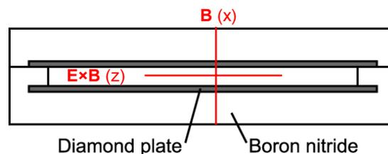
Fig. 2. Schematic of diamond channel design. The red crossbars represent the image of the entrance slit of the streak camera, for the streak images described in the text.
