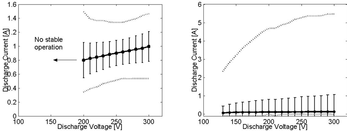
Fig. 6. Oscillation amplitudes of linear Hall thruster. Left: With boron nitride walls. Right: Diamond walls. Error bars indicate the standard deviation of the oscillating current.
