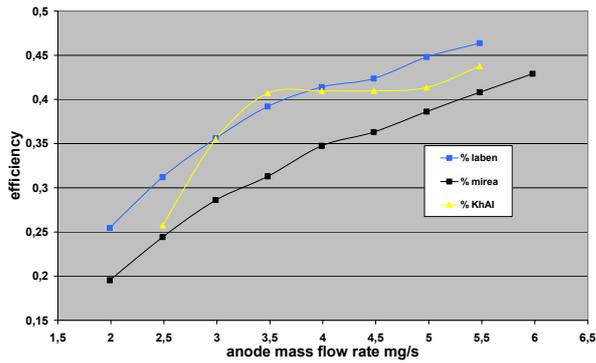
Figure 3: Efficiency as a function of anode mass flow rate (black: MIREA, yellow: KhAI, blue: LABEN)
