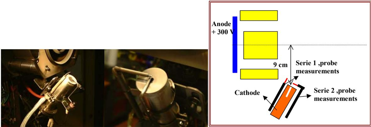
Figure 15: Pictures of the both locations of the electrostatic probes for the hot hollow cathode from MIREA
