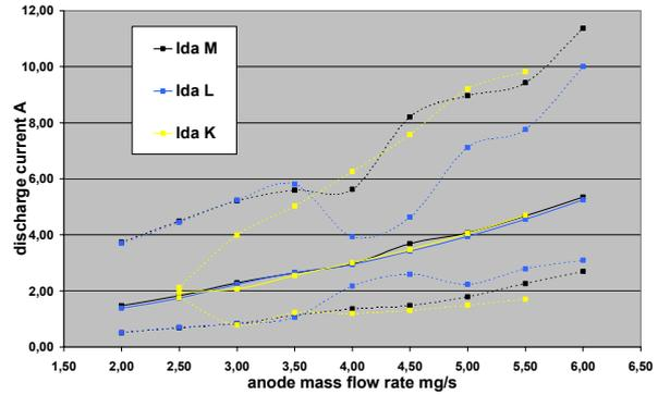
Figure 4: discharge current as function of anode mass flow rate (black: MIREA, yellow: KhAI, blue: LABEN (full lines mean value, dotted lines min & max oscillations))
