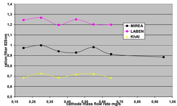
Figure 13 : Ratio CE/CC asymmetry 3 cathodes as function of cathode mass flow rate filter 825nm (neutrals)
