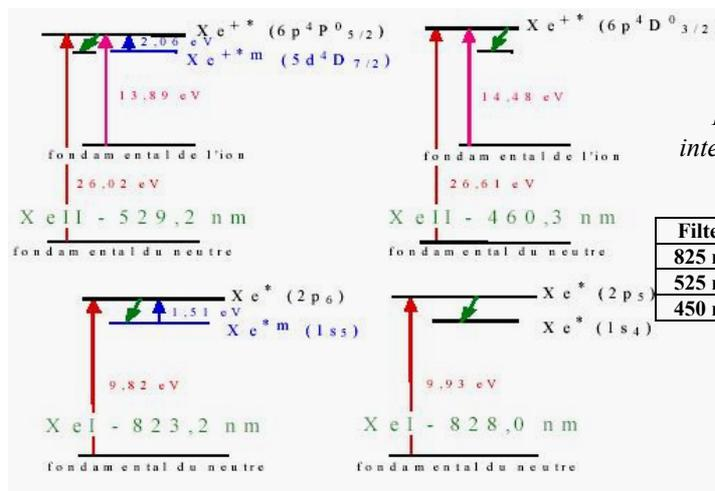
Figure 9: transition lines observed with the interferential filters, top ionic lines, down neutral lines<sup>2</sup>.
