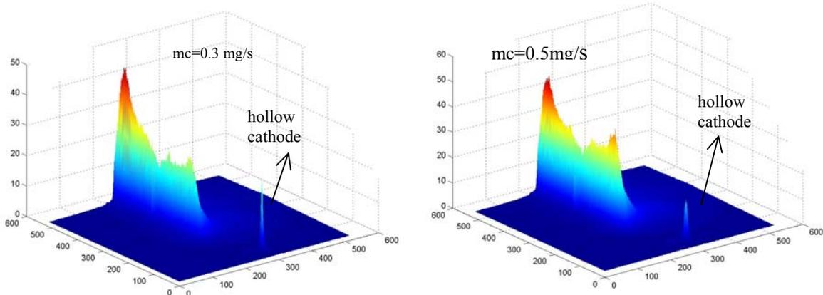
Figure 24: Ion luminous intensity distribution obtained with the CCD camera with a 525 nm filter.
