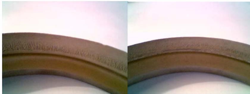
Figure 14 : left: ceramic of the thruster (channel side near the cathode)
