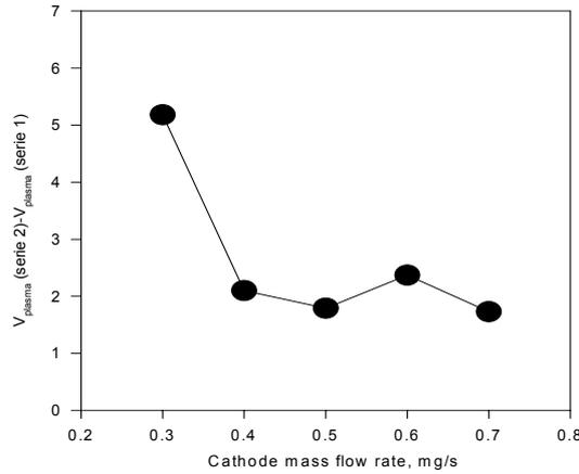
Figure 23 : Difference between the plasma potential for the two series of experiences versus the cathode mass flow rate.
