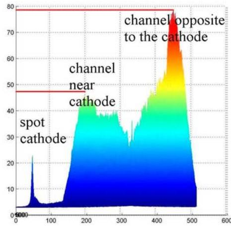
Figure 11: Example of image with the filter at 525nm (ions) taken during the cathode LABEN experiment, treated by MATLAB to observe the asymmetry in the exit plan of the channel.
