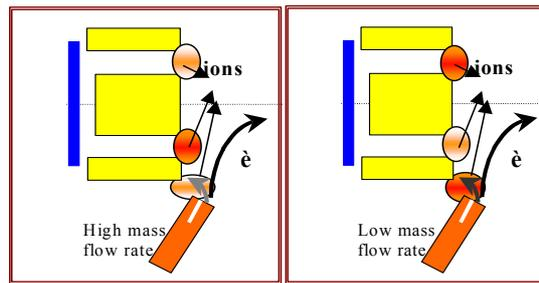
Figure 31: Influence of the cathode mass flow rate on the distribution of ions
