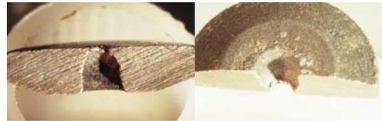
Figure 26: Images given by the KhAI, cutting of the orifice of the cathode. The eroded part faces outside, i.e. towards the spot of light
