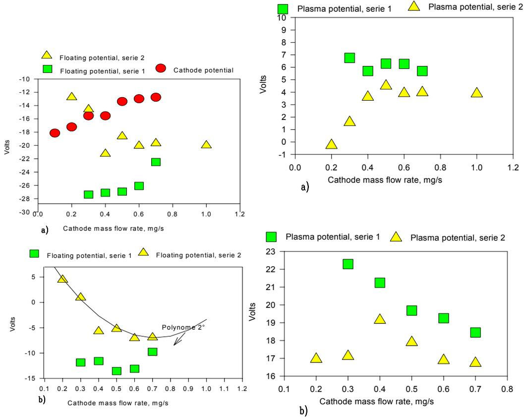
Figure 18: a) floating potential measured relative to the ground; b) floating potential calculated relative to the cathode potential.  $V_d = 300\text{ V}$ ,  $m_a = 5\text{ mg/s}$
