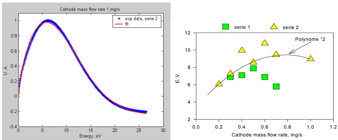
Figure 22: Fit of an experimental EEDF with a Druyvesteyn function.
