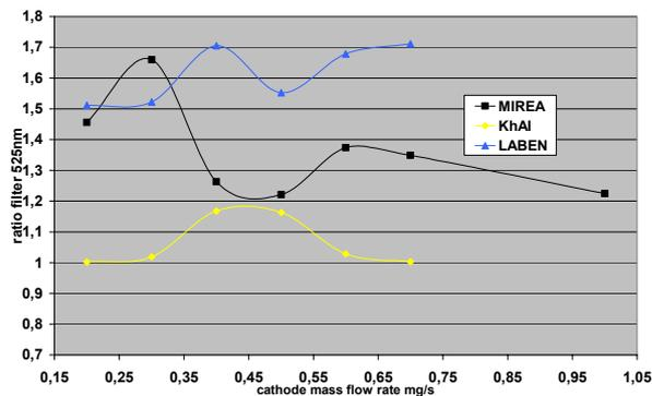
Figure 12 :Ratio CE/CC asymmetry 3 cathodes as function of cathode mass flow rate filter 525nm (ions)
