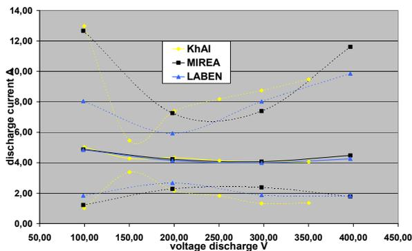
Figure 5: Discharge current as function of discharge voltage (black: MIREA, yellow: KhAI, blue: LABEN full lines mean value, dotted lines min & max oscillations)
