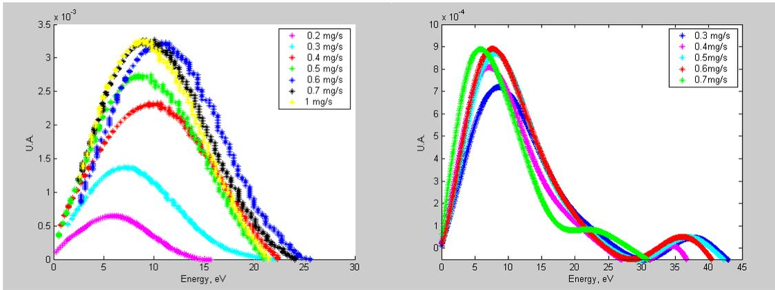
Figure 20: Electron Energy distribution functions at the outlet cathode (serie 2);  $V_d=300$  Volts,  $m_a=5$  mg/s.
