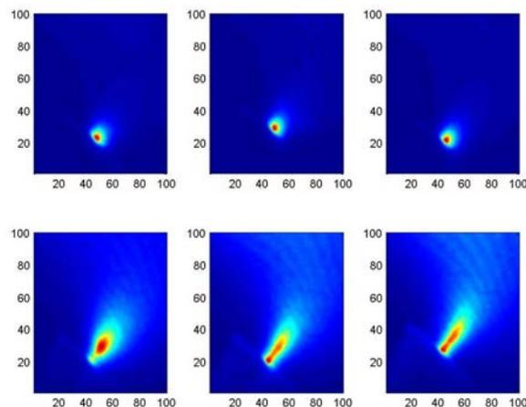
Figure 34: Images of the exit of the orifice, transition mode SPOT/PLUME with the cathode KhAI filter 825nm (neutrals), cathode mass flow rate 0.2, 0.3, 0.4, 0.5, 0.6, 0.7 mg/s with  $m_a=5\text{mg/s}$  and  $V_d=300\text{V}$
