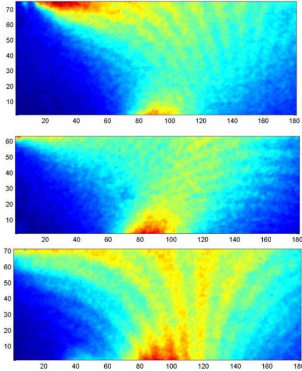
Figure 29: Zone of electronic transport between the cathode and the thruster plume filter 825nm, high :cathode KhAI, scale 1cm->37.5 pixels center cathode LABEN scale 1cm->38.3pixels, down cathode MIREA scale 1cm->28 pixels
