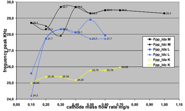
Figure 8: frequency Main peak of discharge current (picked up on the anode line and on the cathode line) as function of cathode mass flow rate
