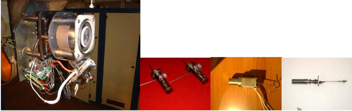
Figure 1: Photograph of the SPT100-ML in the PIVOINE facility with two electrostatic probes: beside the body of the cathode and close to the exit plane of the thruster (top).
