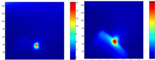
Figure 25: Image of MIREA cathode spot,  $m_c=0.4\text{mg/s}$ ,  $m_a=5\text{mg/s}$ ,  $V_d=300\text{V}$  1) filter 525nm ions 2) 825nm neutrals
