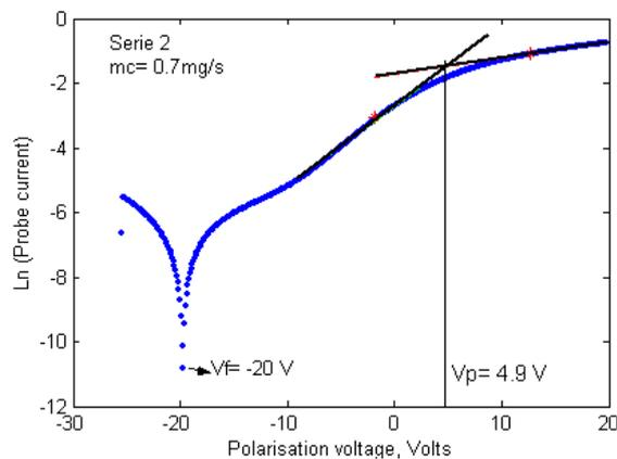
Figure17: Probe characteristic obtained for the serie 1
