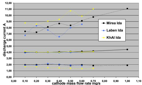
Figure 6 : discharge current as function of cathode mass flow rate (full lines mean value, dotted lines max & min limits of observed oscillations)
