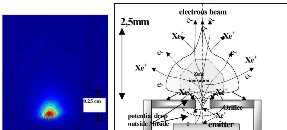
Figure 27: Zoom on luminous spot, filter 525nm ions, and iso intensity lines, scale of image gives size about 2.5mm of height.
