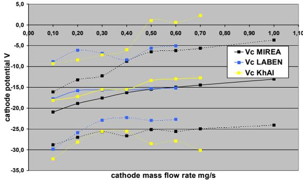
Figure 7: cathode potential as function of cathode mass flow rate (full lines mean value, dotted lines max & min of oscillations)
