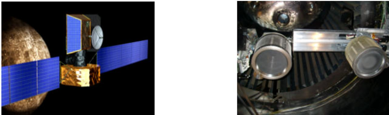
**Figure 5.** A candidate configuration for the BepiColombo spacecraft to Mercury and two T6 candidate Ion Thrusters undergoing twin firing test at QinetiQ (UK).
