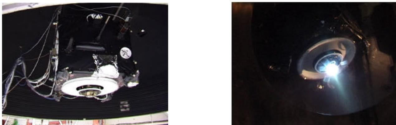
**Figure 4.** The SMART-1 spacecraft mounted in the end-to-end test facility at ESTEC (left) and the PPS-1350 thruster firing during the test (right)
