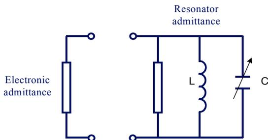
**Figure 5. Plasma as a 'two-terminal' oscillator**
