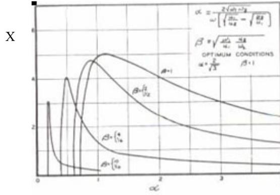
Figure 8. Plot of wave Gain factor X against  $\alpha$
