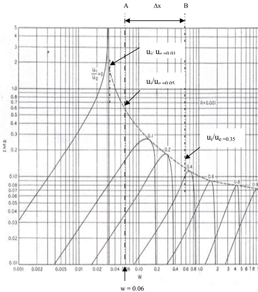
**Figure 7. Wave gain parameter  $Imz$  against  $W$  the ratio of signal frequency to electron plasma frequency.**
