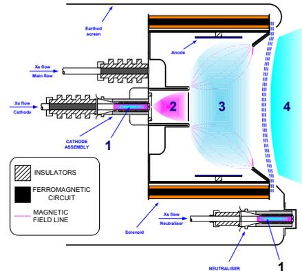
Figure 2. Various plasmas in UK10 Ion thruster
