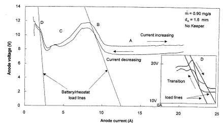
**negative conductance of a hollow cathode plasma.**
