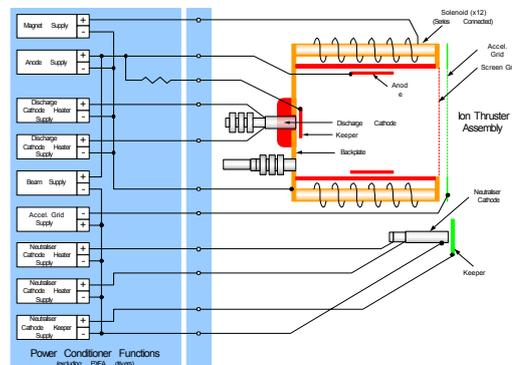
Figure 3. Various closed electrical-loop circuits in an electrostatic ion thruster
