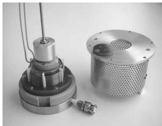
Figure 18. Photograph of the disassembled Giessen microthruster RIT-4.
