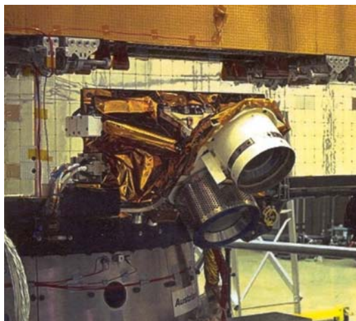
Figure 6. Package of two EP-engines (RITA and EITA) onboard ESA's advanced communication satellite ARTEMIS.
