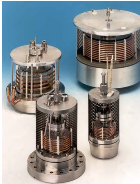
Figure 11. Radio-frequency ion engines for material processing (RIM-family) with 4 cm and 6 cm diam (company Pfeiffer) and with 10 cm and 20 cm diam (Giessen University, 1988).
