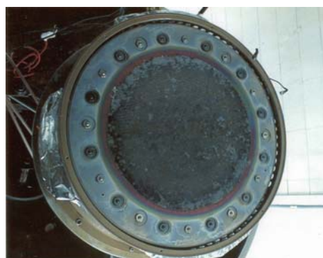
Figure 9. The 26 cm rf-ion engine ESA-XX (main contractor Dasa) after performance tests in the large Giessen test stand (1994).
