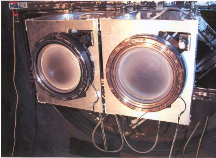
Figure 10. Two RIT-22 thrusters of EADS Space Transportation tested in the 30 m 3 vacuum facility of Giessen University (2004).
