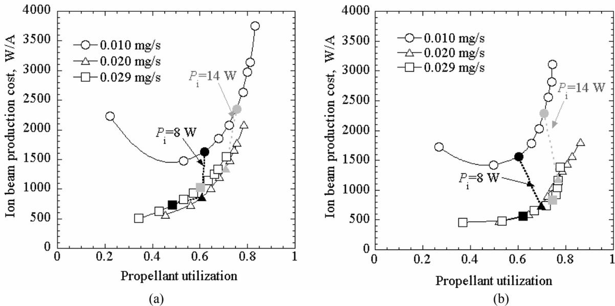
Figure 7. Thrust performance of star antenna for three levels of ion production.
