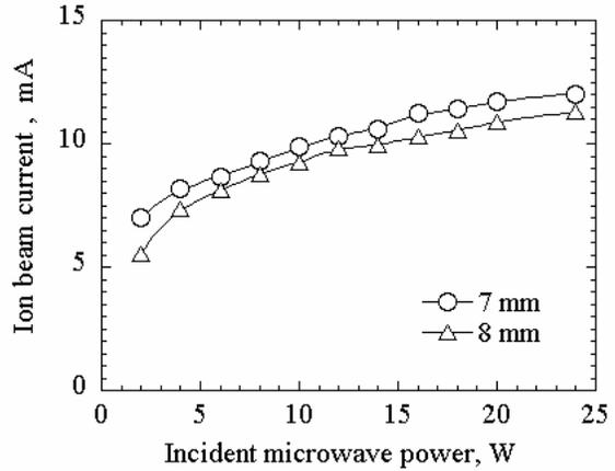
Figure 6. Thrust performance of star antenna.
