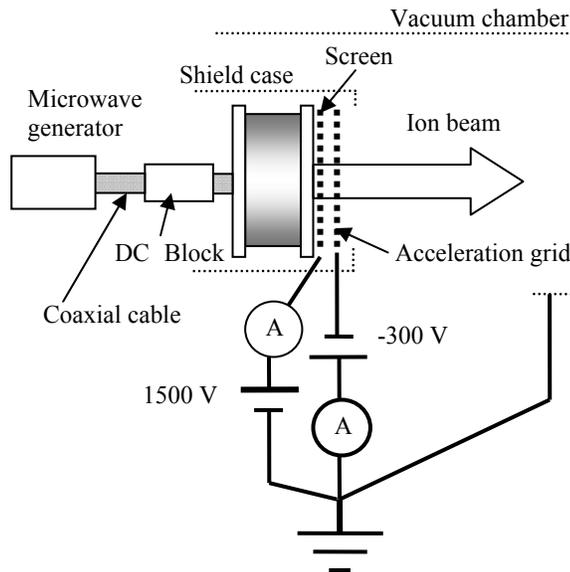
**Figure 4. Schematic of electric circuit.**
