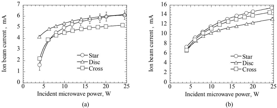
**Figure 5. Thrust performance for different levels of ion production.**
