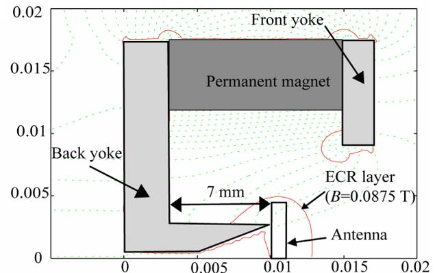
Figure 2. Magnetic field profile of miniature ion engine.
