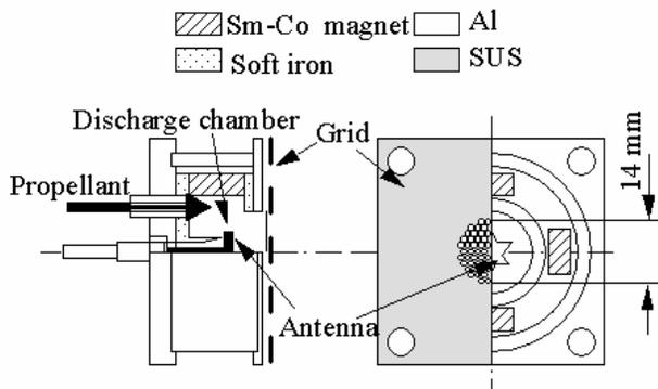
Figure 1. Cross-section of miniature ion engine developed at Kyushu University.
