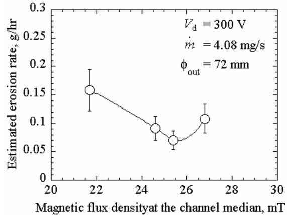
Figure 10. Relation between erosion rate and magnetic flux density.
