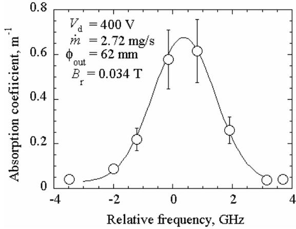
Figure 8. Absorption profile of target spectrum.
