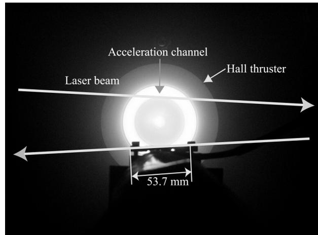
**Figure 4. Appearance of Hall thruster operation.**
