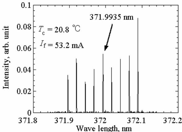
Figure 6. Spectrum of ultra violet laser diode. at  $I_f=53.2$  mA.
