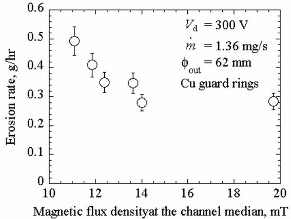
Figure 5. Relation between erosion rate and magnetic flux density by duration test.
