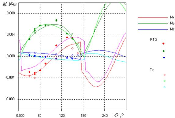
Figure 10 Comparison of calculated torque with *Express* data for  $T3$ ,  $RT3$
