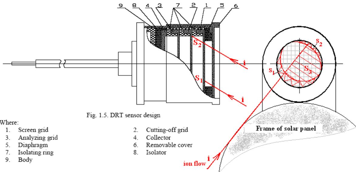
**Figure 2 DRT sensor design and the shape of shading ( $S_1, S_2, S_3$ ) of grides by structure elements of the sensor and the frame**
