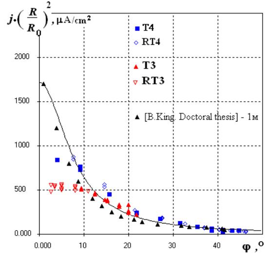
**Figure 5. Angular dependence of current density. Theoretical model (4) - solid curve. Experimental data -symbols- are normalized to 1m with use of conical approach (4)**
