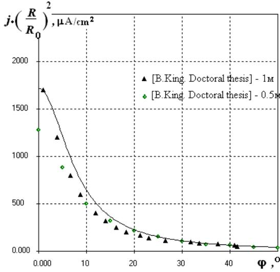
**Figure 4 Experimental [4] and theoretical (4) angular dependencies of ion current density of the SPT-100 plume**
