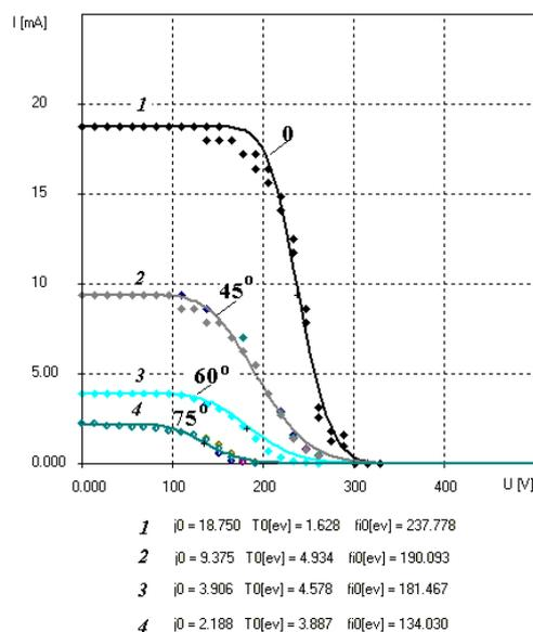
**Figure 8 Change of braking characteristics with reference to angular position of the sensor**
