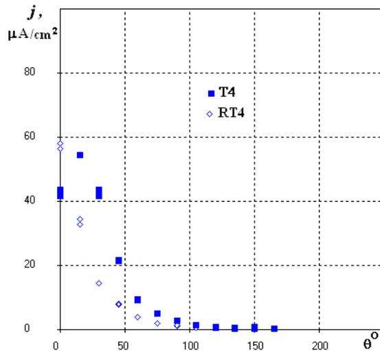
**Figure 3 Dependence of ion current density  $j$  versus solar panel rotation  $\theta$ . Data are measured by DRT1 at operation of  $T4$  and  $RT4$  thrusters**
