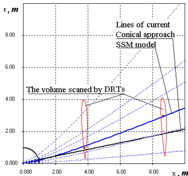
**Figure 7 Comparison between a conical approach and SSM model with reference to the plume of SPT-100 on “Express” satellite**
