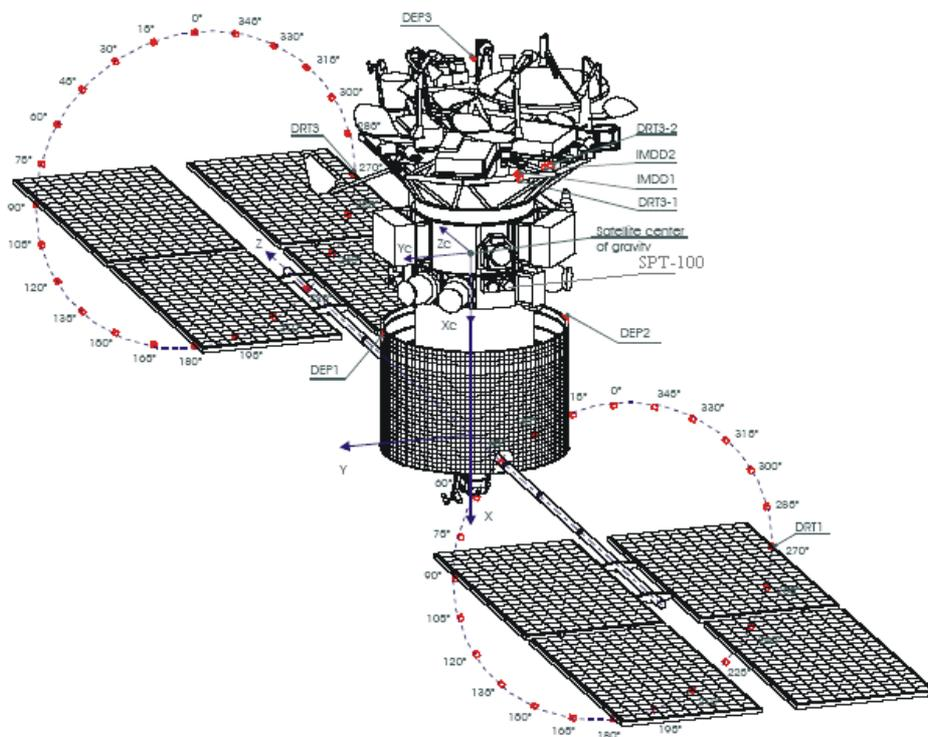
Figure 1 General view of "Express" satellite and dislocation of the SPT-100 thrusters and DRT sensors.
