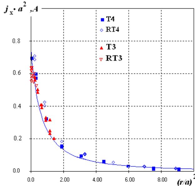
**Figure 6 Angular dependence of current density. SSM model - solid curve. Experimental data –symbols– are normalized to 1m with use the SSM model**
