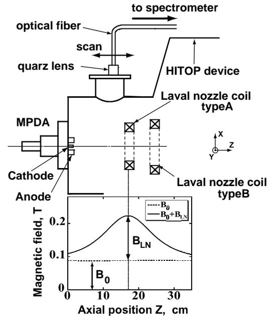
Figure 3. Layout of alternatively used two types of Laval-nozzle coils. Axial profiles of the magnetic field near the MPDT are shown in case of type-A coil ( $B_{LN}$ ) in addition to a uniform field ( $B_0$ ).
