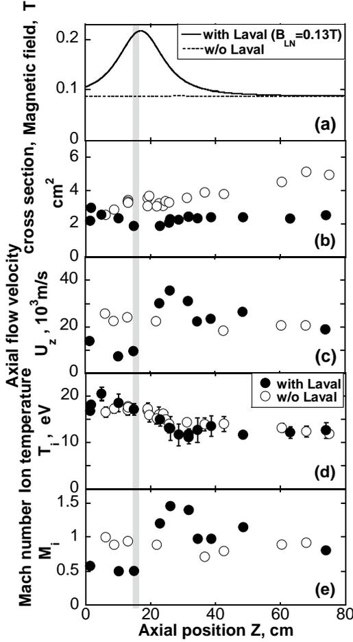
Figure 7. Axial profiles of (a)  $B_z$ , (b) plasma cross section measured by spectroscopy  $A$ , (c)  $U_z$ , (d)  $T_i$ , and (e)  $M_i$ , with and without the type-A magnetic Laval nozzle coil.  $I_d=7.2\text{kA}$ ,  $B_0=0.087\text{T}$ .
