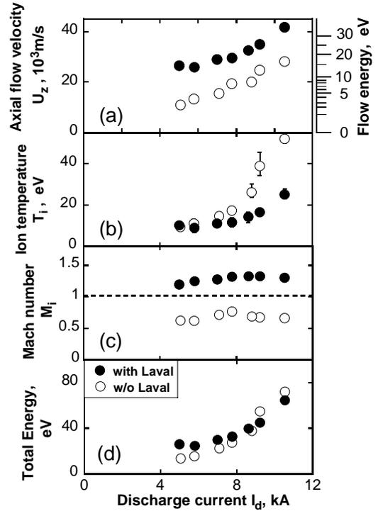
Figure 5. Flow characteristics with (solid circles) and without (open circles) the Laval nozzle as a function of discharge current of the MPDT measured in the downstream region of the Laval nozzle ( $Z=30.5\text{cm}$ ).
