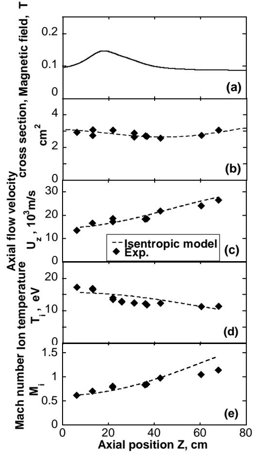
Figure 8. Same as in Fig.7 using the type-A and B Laval nozzle coils. Dotted lines corresponds to predicted value by 1-D isentropic flow model.
