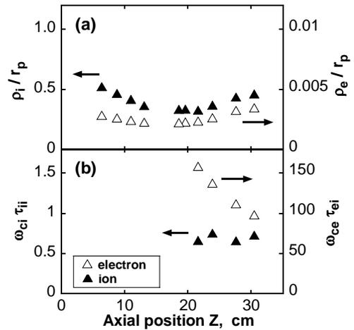
Figure 6. Axial profiles of (a) ratios of a Larmour radius to a plasma radius,  $\rho_e/r_p$  and  $\rho_i/r_p$ , and (b) Hall parameters,  $\omega_{ce}\tau_{ee}$  and  $\omega_{ci}\tau_{ii}$ , for electrons and ions.
