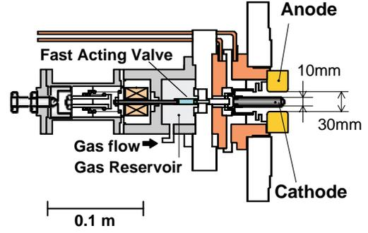
Figure 2. A side view of the MPD thruster.
