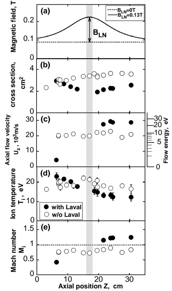
Figure 4. Axial profiles of flow characteristics with (solid circles) and without (open circles) the Laval nozzle. A subsonic flow is converted into a supersonic one passing through the magnetic Laval nozzle.  $I_d=7.2\text{kA}$ .
