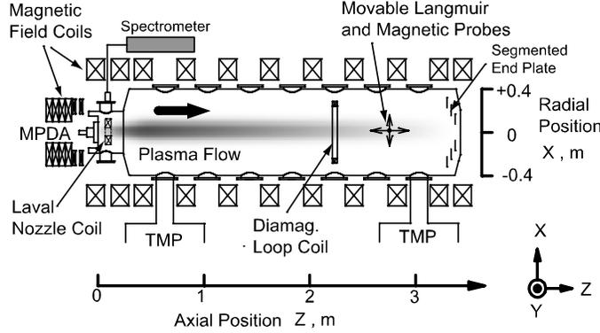
Figure 1. Schematic view of the HITOP device.
