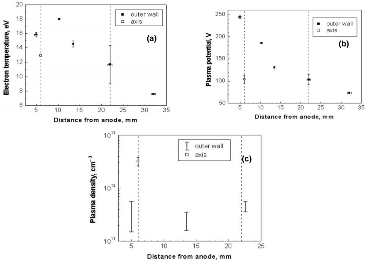
Fig. 3. Electron temperature (a), plasma potential (b), and plasma density (c) profiles in the 2.6 cm CHT.<sup>28</sup> Dashed lines at  $z=6$  mm and  $z=22$  mm show the edge of the annular channel part and the thruster exit, respectively. In (a) and (b), Y-axis error bars represent the entire statistical spread of the measured data. For plasma density measurements near the outer channel wall (c), only the intervals, in which the real values of the plasma density are located, can be given.
