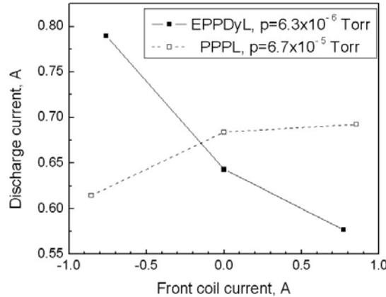
Fig. 3. The dependences of the discharge current on the current in the front magnetic coil in the 2.6 cm CHT for the EPPDyL and PPPL facilities. All discharge parameters are the same (anode flow rate  $\mu=0.4$  mg/s,  $U_d=250$  V,  $I_{back}=+3$  A), except for the background gas pressure, which is equal to  $6.3 \times 10^{-6}$  Torr for the EPPDyL tank and  $6.7 \times 10^{-5}$  Torr for the PPPL tank.
