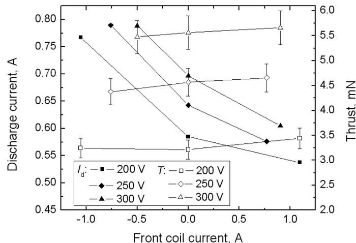
Fig. 4. The dependences of the discharge current and thrust on the front coil current in the 2.6 cm CHT operated in the EPPDyL facility (background gas pressure  $\sim 6 \times 10^{-6}$  Torr). Anode and cathode xenon flow rates are 4 sccm and 2 sccm, respectively;  $I_{back} = 3$  A.  $I_{front} > 0$  ( $I_{front} < 0$ ) corresponds to the direct (cusp) magnetic field configuration.
