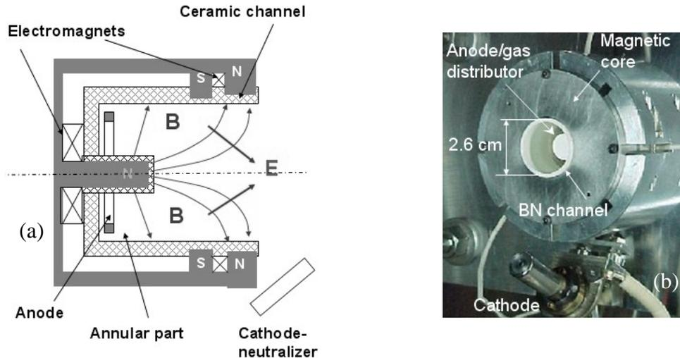
Fig. 1. (a) Schematic of a cylindrical Hall thruster. (b) The 2.6 cm cylindrical Hall thruster.
