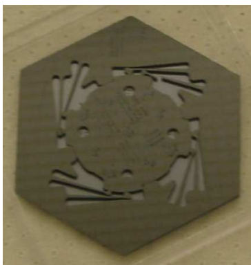
Figure 9. An assembled grid with a broken finger.
