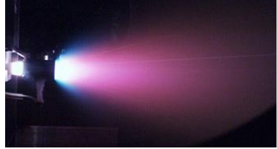
Figure 5. Photograph of firing PPT (PTFE, cavity length: 14 mm, Stored energy=21.4J).
