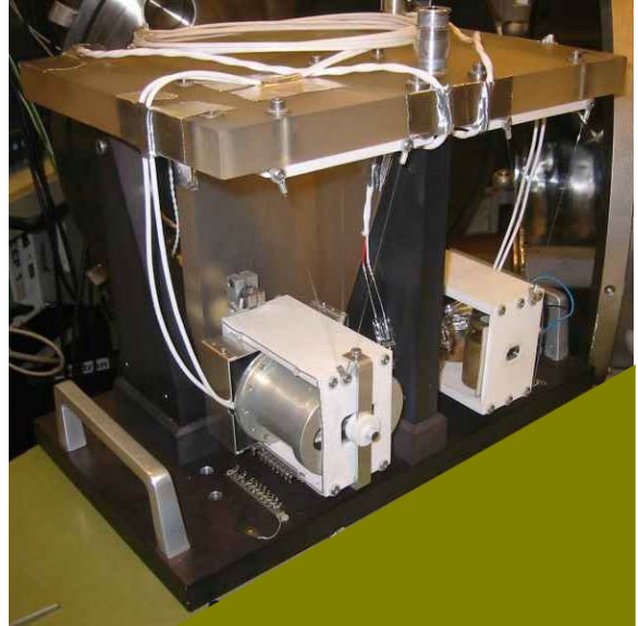
Figure 6. FEEP micro-thrust balance integrated with a FEEP thruster on the left side. The high voltage power feeding cables are visible (2 on each side).
