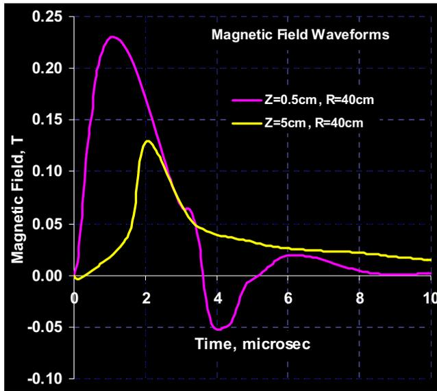
**Figure 12. Radial Magnetic Field waveforms computed by MACH2 at a radial location of  $40\text{cm}$  and axial locations of  $0.5\text{cm}$  and  $5\text{cm}$ .  $E_0=1764\text{J}$ ,  $m=2.1\text{mg}$ .**
