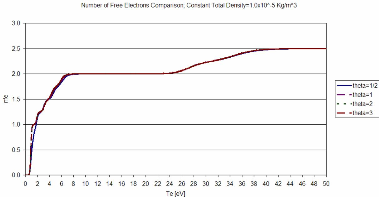
**Figure 8. Number of free electrons per heavy particle, (average charge) as a function of electron temperature and varying temperature ratio,  $\theta=T_e/T_h$  at  $\rho=10^{-5}$  kg/m<sup>3</sup>.**
