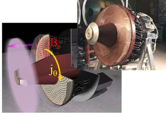
**Figure 1. The Pulsed Inductive Thruster (PIT) (Courtesy NGC) and a schematic of the main acceleration process due to the interaction of the applied radial field and the induced azimuthal current.**
