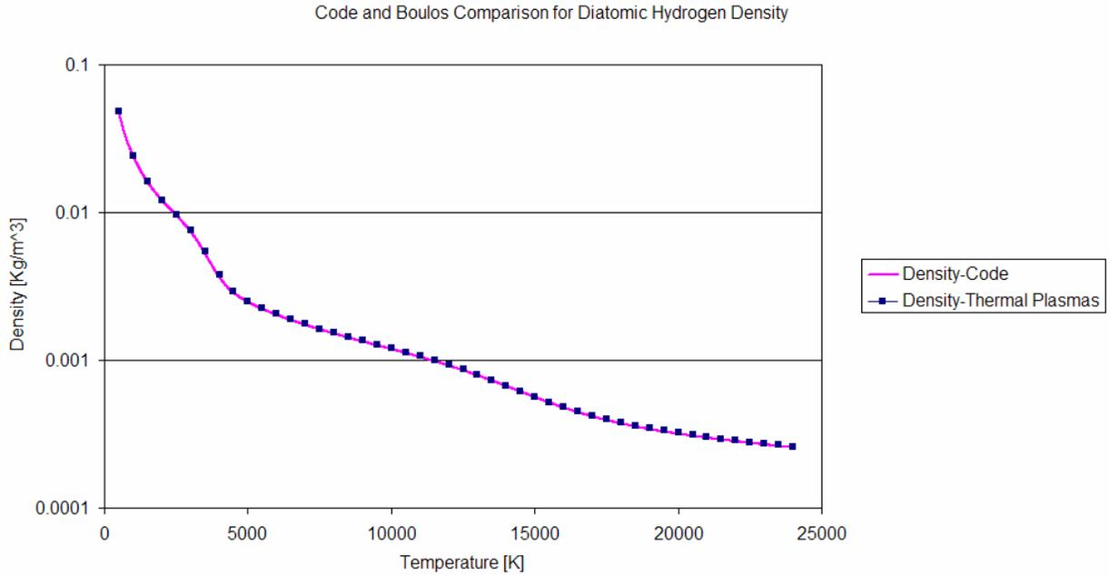
**Figure 6. Comparison of the code's computed density profile as a function of temperature, (equation of state) to Boulos' model for hydrogen at 100kPa.**
