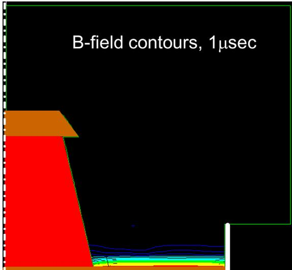
Figure 13. Magnetic Field contours for  $\text{NH}_3$  at 1  $\mu\text{sec}$ .  $E_0=1764\text{J}$ ,  $m=2.1\text{mg}$ .
