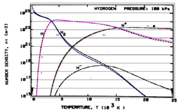
Figure 2. Comparison of hydrogen composition predicted by the code (solid colored) to Boulos' as a function of temperature.
