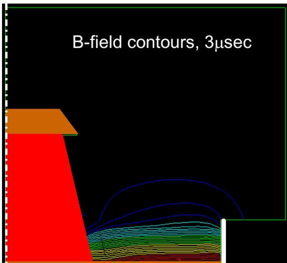
Figure 15. Magnetic Field contours for  $\text{NH}_3$  at 3  $\mu\text{sec}$ .  $E_0=1764\text{J}$ ,  $m=2.1\text{mg}$ .
