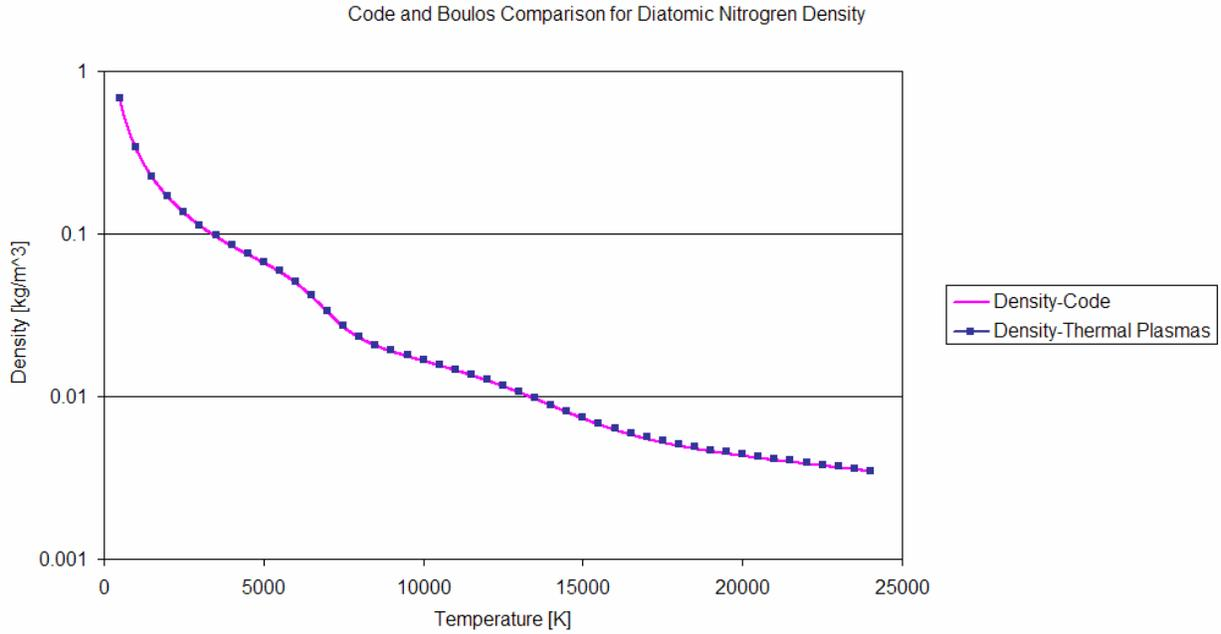
**Figure 4. Comparison of the code's computed density profile as a function of temperature, (equation of state) to Boulos' model for nitrogen at 100kPa.**
