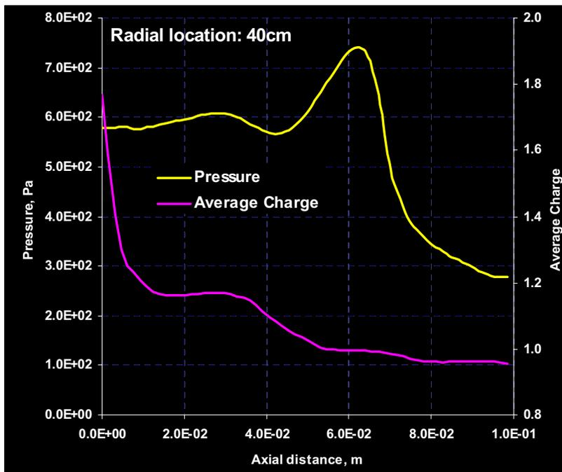
Figure 17. Plasma Pressure and Average degree of Ionization profiles as a function of axial distance,  $z$  at  $10\mu\text{sec}$ .  $E_0=1764\text{J}$ ,  $m=2.1\text{mg}$ .
