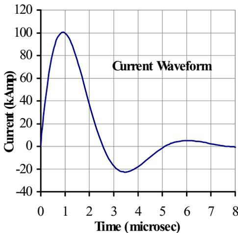
**Figure 11. MACH2 calculated Current Waveform used to emulate the PIT's circuitry,  $V_{eff} = 28kV$ .**
