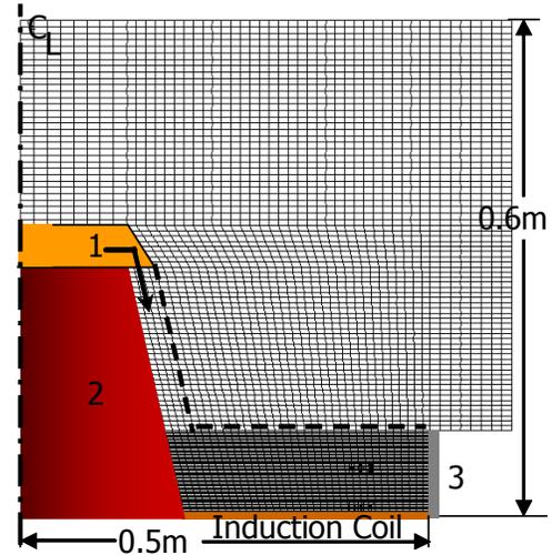
**Figure 10. Schematic of the half-plane thruster with the computational grid utilized, (not to scale). 1: Nozzle with pulsed mass-valve, 2: Conical pylon, 3: Confining cuff (lexan).**
