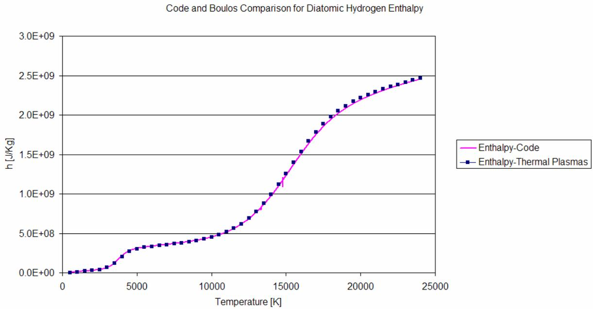
**Figure 7. Comparison of the code's computed enthalpy profile as a function of temperature, (caloric equation of state) to Boulos' model for hydrogen at 100kPa.**
