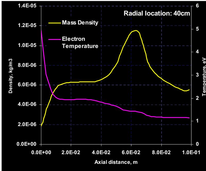
Figure 16. Mass Density and Electron Temperature profiles as a function of axial distance,  $z$  at  $10\mu\text{sec}$ .  $E_0=1764\text{J}$ ,  $m=2.1\text{mg}$ .
