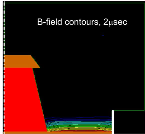
Figure 14. Magnetic Field contours for  $\text{NH}_3$  at 2  $\mu\text{sec}$ .  $E_0=1764\text{J}$ ,  $m=2.1\text{mg}$ .
