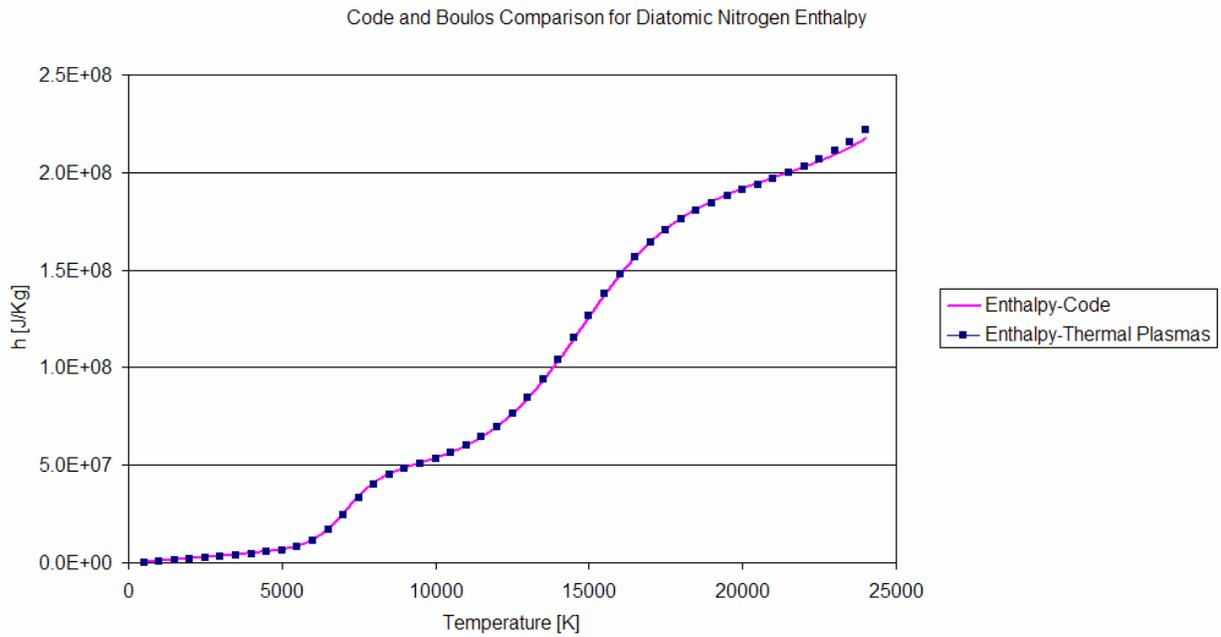
**Figure 5. Comparison of the code's computed enthalpy profile as a function of temperature, (caloric equation of state) to Boulos' model for nitrogen at 100kPa.**
