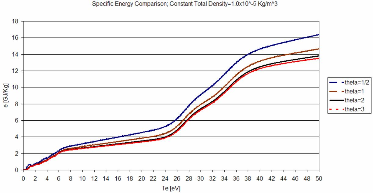
**Figure 9. Specific internal energy as a function of electron temperature and varying temperature ratio,  $\theta = T_e/T_h$  at  $\rho = 10^{-5}$  kg/m<sup>3</sup>.**
