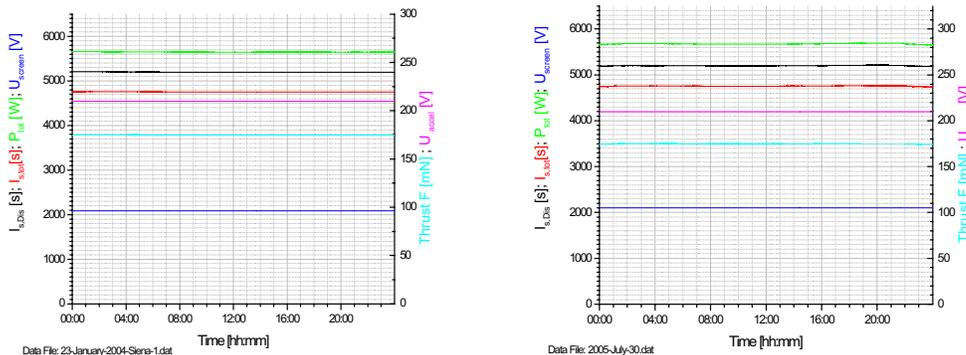
**Figure 9** Typical daily data sheets from the 3.000h endurance test with the RIT-22 Ion Engine: Left January 2005, right: July 2005, last day before switching-off the engine for 3.000h grid inspection
