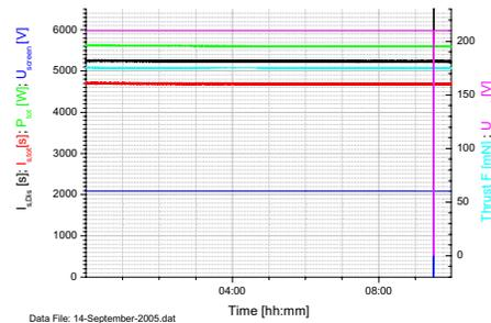
The test is performed in the Giessen University Jumbo Test Facility (for details see ref [16]). In the meantime the first two segments were completed and the third segment is ongoing. Although the two test facilities, Giessen University and Aerospazio Technologies are different w.r.t. size, equipment and pumping concept, the engine shows up to now the same stability an performance in the much smaller Giessen test chamber.
