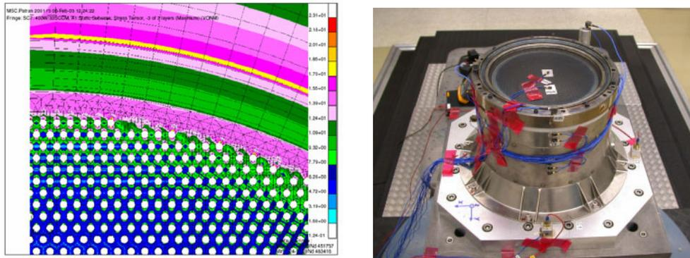
**Figure 7** FEM Analysis of the grid system (accelerator) and grid system mounted on RIT-22 ion engine after vibration test
