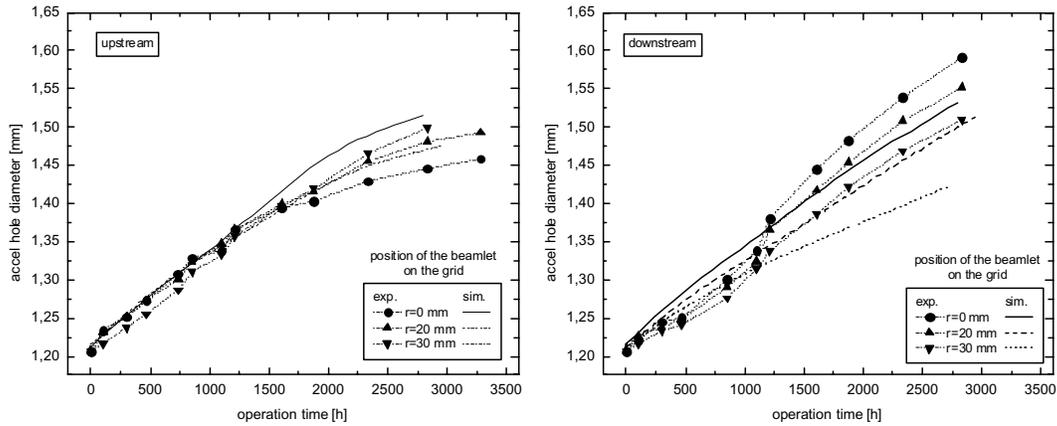
**Figure 4** Evolution of the accelerator grid hole diameters upstream (left) and downstream (right), comparison of measured and simulated data.
