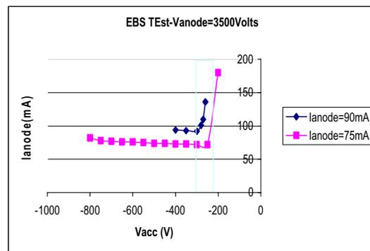
**Figure 13.** EBS Test with High Specific Impulse Ion Optics
