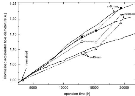
Figure 7: Evolution of the accelerator grid hole diameters (normalised to 1.0 at 3.000 h) with time in comparison with lifetest results.
