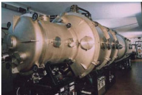
**Figure 12** Alenia-Laben vacuum test facility for ion thruster endurance test
