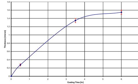
**Figure 3** Deposited thickness for different process durations: a saturation phenomenon, probably due to the insulating behavior of the layer, is clearly present preventing the thickness from reaching higher values
