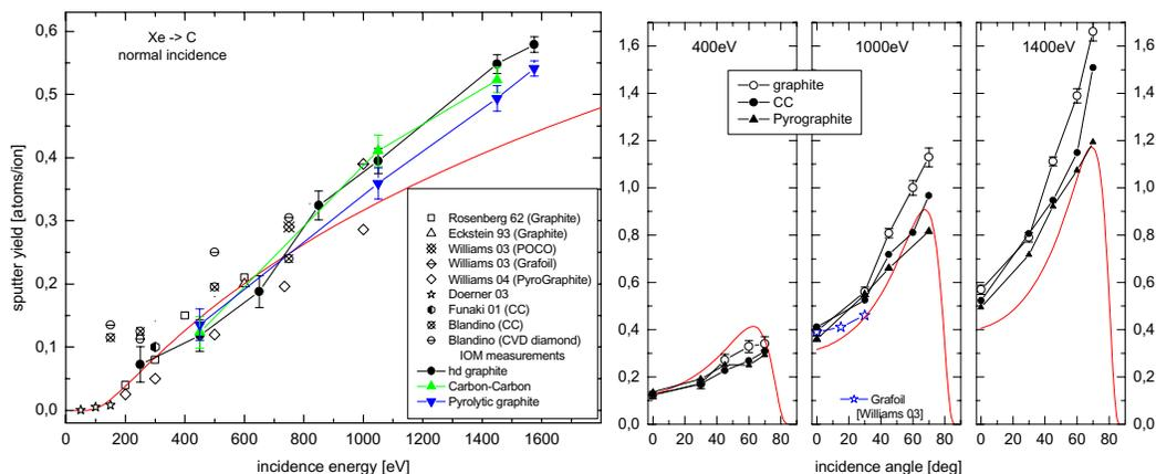
**Figure 1** Sputter yields of graphite, Carbon-Carbon and pyrolytic graphite in dependence on xenon ion energy and angle. Solid lines are the semi-empirical sputter models of Bohdansky and Yamamura.
