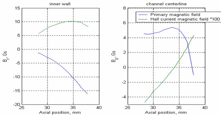
**Figure 5. The comparison of the primary magnetic field and Hall current magnetic field in the region where the sensors may be placed.**
