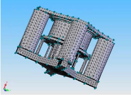
**Figure 10. Thermal model meshing**
