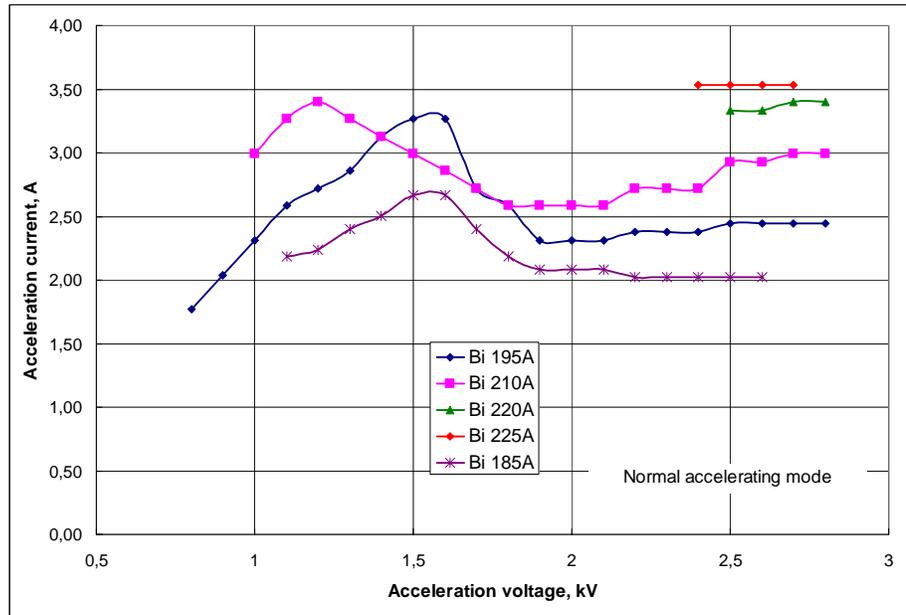
**Figure 18. D-160 Volt-ampere characteristics**
