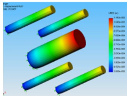
**Figure 13. The disposition and value of absolute displacements of the central and side coil free faces**
