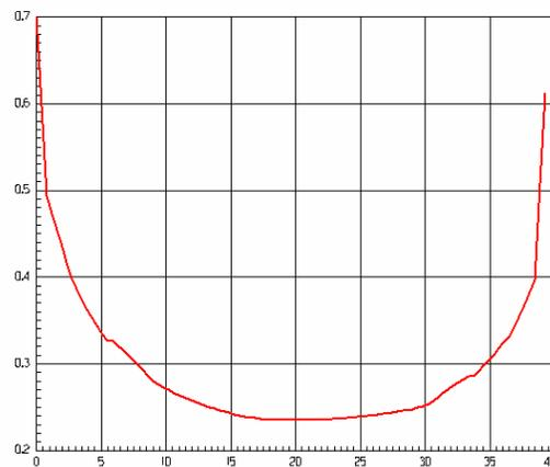
**Figure 6. Magnetic field distribution along radius in the gap between the pole centers**
