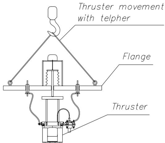
**Figure 14. Scheme of moving the thruster mounted on the flange**
