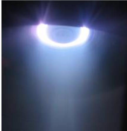
**Picture 7. D-160 discharge and plume**
