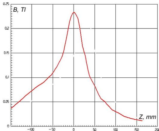
**Figure 5. Magnetic field distribution along accelerating channel axis**
