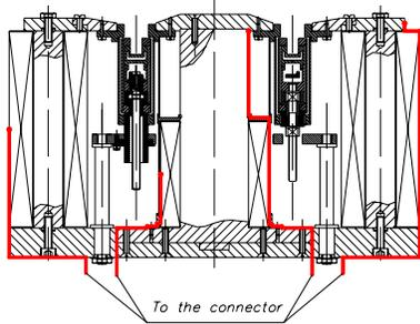
**Figure 16. The thermocouples installment points and its layout**
