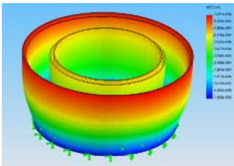
**Figure 12. The disposition and value of absolute displacements of the thermal screen free faces**
