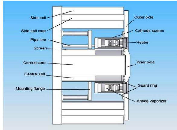
**Figure 9. Elements of the thruster thermal model**
