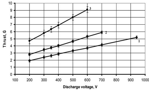
**Figure 2. The dependence of the thrust from the discharge voltage (A-5).**
