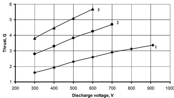
**Figure 5. The dependence of the thrust from the discharge voltage (A-3).**
