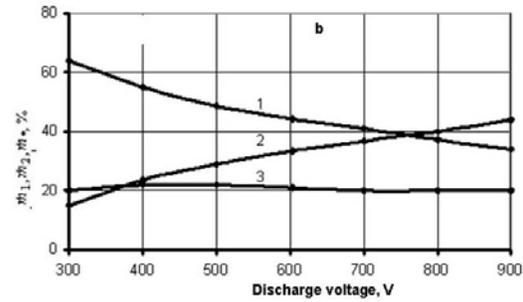
**Figure 9. SPT A-3.** The dependence  $\dot{m}_1$  (1),  $\dot{m}_2$  (2),  $\dot{m}_*$  (3) of  $U_d$   $\dot{m}=1$ mg/s. Flows are given in percent accordance with mass flow rates.
