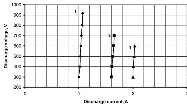
**Figure 4. The dependence of the discharge current from the discharge voltage (A-3).**
