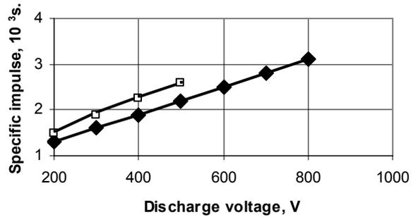
**Figure 3. The dependence of the specific pulse from the discharge voltage (A-5).**
