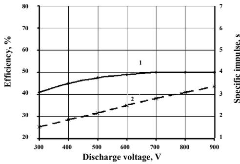
**Figure 8. Integral parameters of SPT A-3.** The dependence of efficiency ( — ) and specific impulse ( - - - ) from the  $U_d$   $\dot{m}=1$  mg/s.
