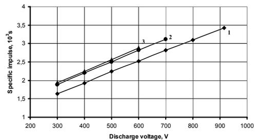
**Figure 6. The dependence of the specific impulse from the discharge voltage (A-3).**
