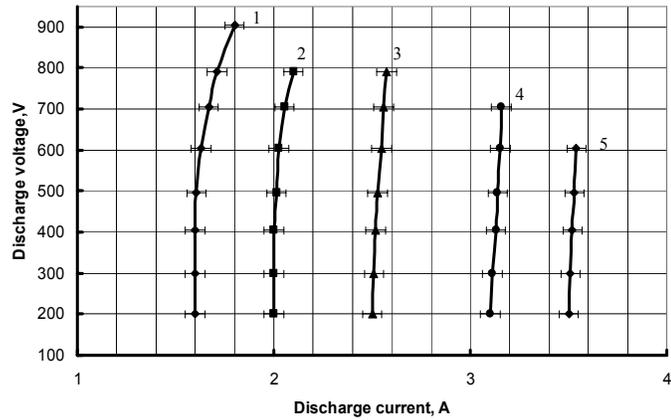
**Figure 1. The dependence of the discharge current from the discharge voltage (A-5). 1 -  $\dot{m} = 1,5 \text{ mg/s}$ , 2 -  $\dot{m} = 2 \text{ mg/s}$ , 3 -  $\dot{m} = 2,5 \text{ mg/s}$ , 4 -  $\dot{m} = 3 \text{ mg/s}$ , 5 -  $\dot{m} = 3,5 \text{ mg/s}$ .**
