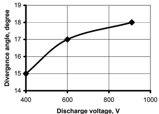
**Figure 7. The graph of the half-angle of the divergence  $\alpha/2$  versus discharge voltage  $U_d$  (A-3)**
