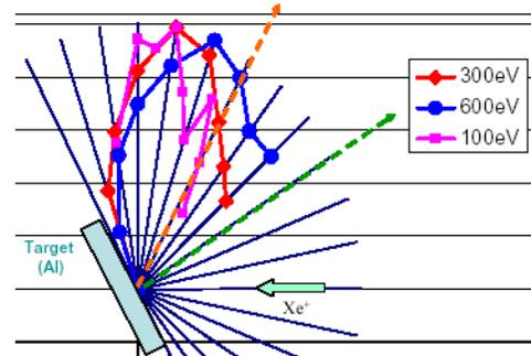
**Figure 6. Example of an emission profile of Aluminum sputtered by a Xenon ion flux<sup>17</sup>**
