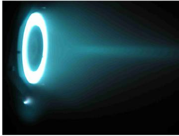
**Figure 5. PPS-X000 technological demonstrator in operation**
