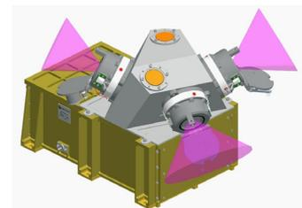
Figure 11. Electric Propulsion Subsystem Assembly – pre-PDR design
