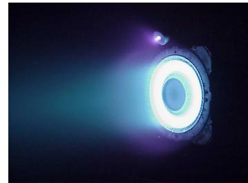
Figure 3. PPS-1350-G thruster in operation
