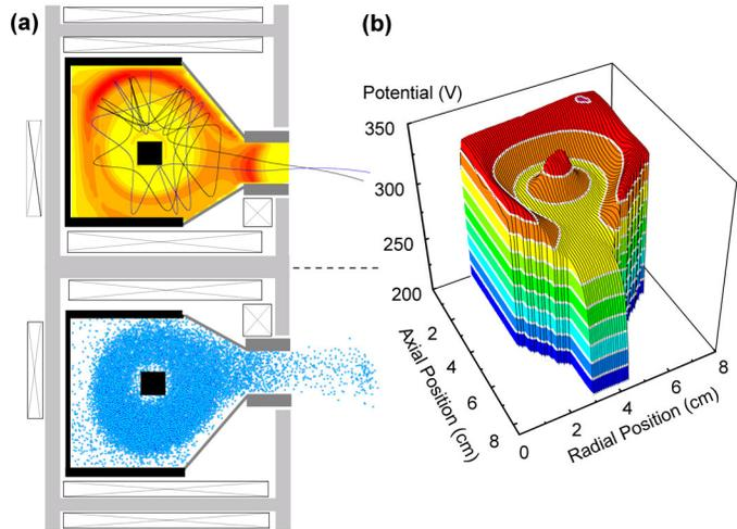
Figure 1. Numerical simulation of a double-stage plasma thruster (left: ionization rate (top) and ion location (bottom) ; right: potential)<sup>8</sup>
