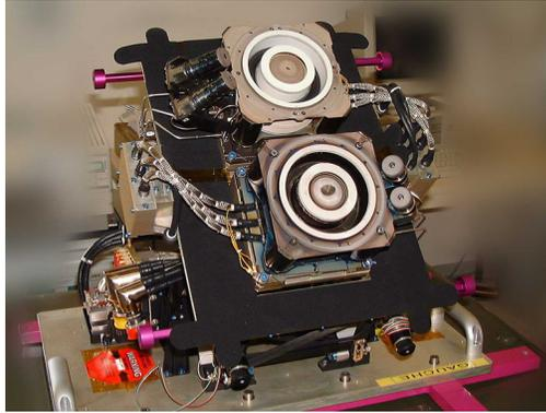
**Figure 7. STENTOR electric propulsion module made of one SPT-100 and one PPS-1350 thrusters mounted on an ALCATEL gimbals mechanism.**
