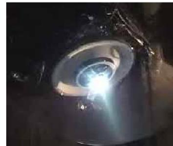
**Figure 8. SMART-1 PPS-1350 thruster in operation on the spacecraft during end-to-end tests<sup>19</sup>**
