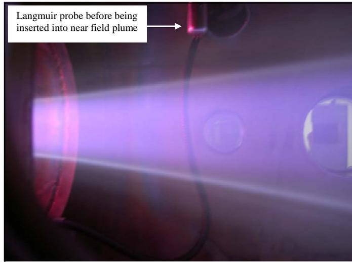
**Figure 2. Near field plume of a thruster with a diagnostics parked near plume**
