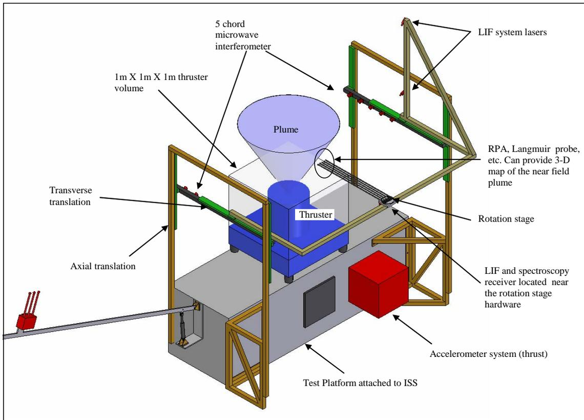
**Figure 3. Conceptual layout of near field plume diagnostics**
