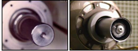
Fig 1. NSTAR hollow cathode at the beginning (left) and end (right, 30,352 hrs) of the Extended Life Test.
