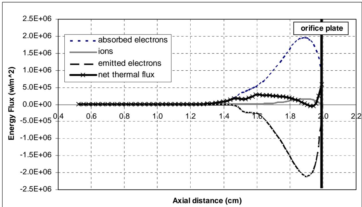
Fig 5. Components of the plasma energy flux to the insert emitter surface.
