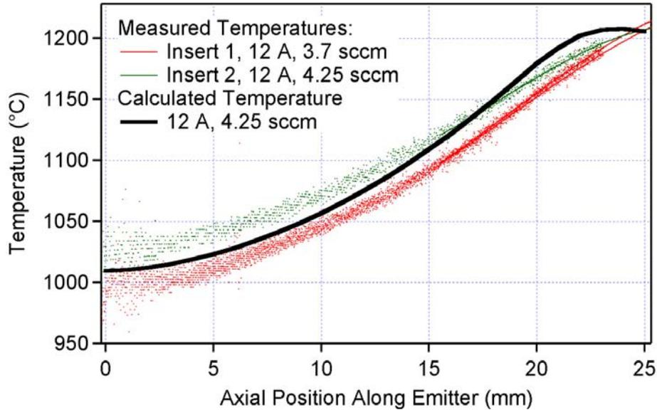
Fig 7. Measured emitter temperatures. The HCThermal calculation was performed for Insert 2.
