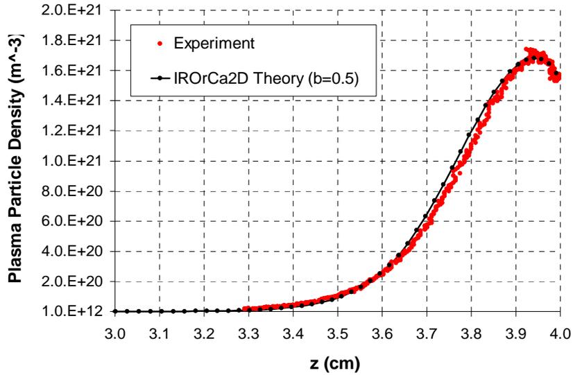
Fig 3. Comparison between measurement and theory (using the IROrCa2D code) for the plasma particle density along the axis of symmetry of the NSTAR cathode. Emission enhancement (with an enhancement factor  $b=0.5$ ) and emission turn-off are both included in the IROrCa2D result.
