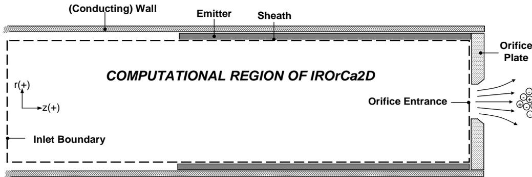
Fig 1. Hollow cathode emitter region schematic showing the region modeled by IROrCa2D.
