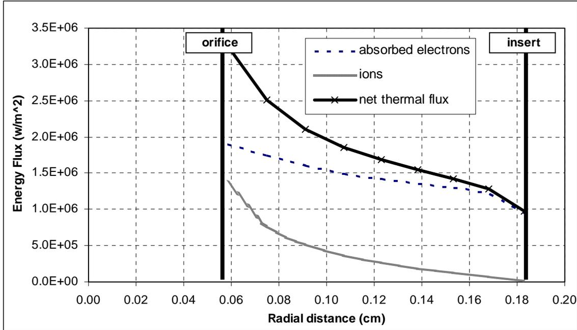
Fig 6. Components of the plasma thermal flux to the upstream surface of the orifice plate.
