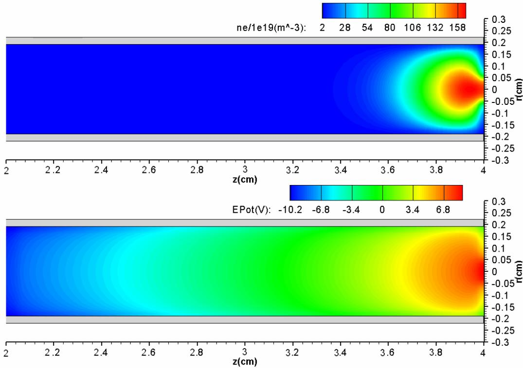
Fig 4. IROrCa2D computed profiles of the plasma particle density (top) and plasma potential (bottom).
