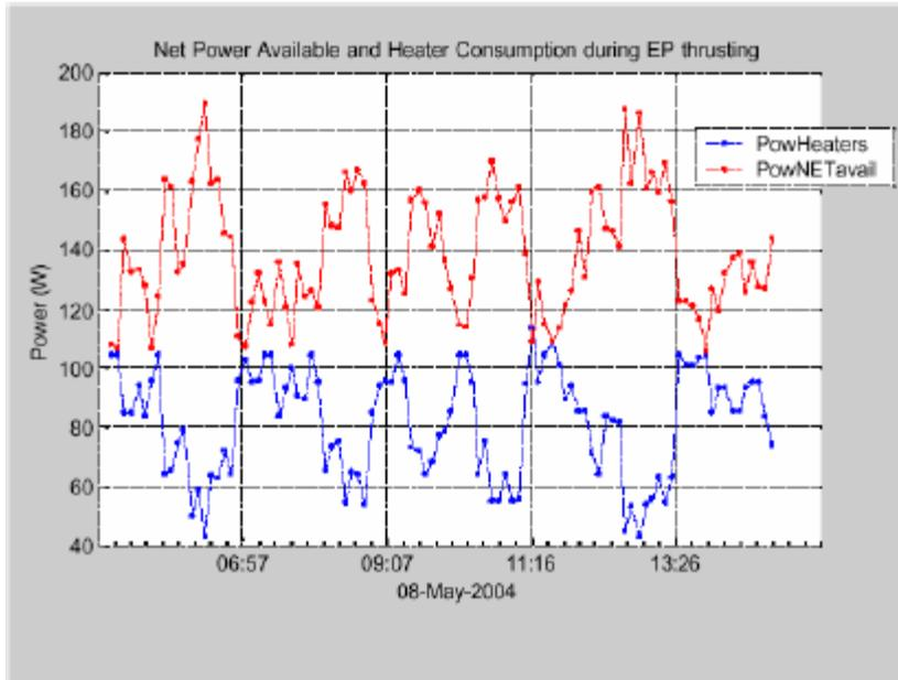
**Figure 2 Total Heater Power Consumption, and overall instantaneous net available onboard power**
