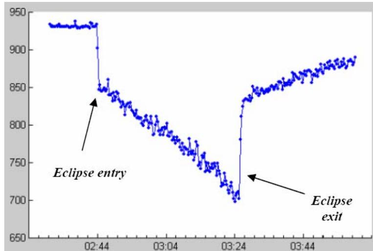
**Figure 5 An example Battery Charge Status (Whrs) through an eclipse (SMART-1 data)**
