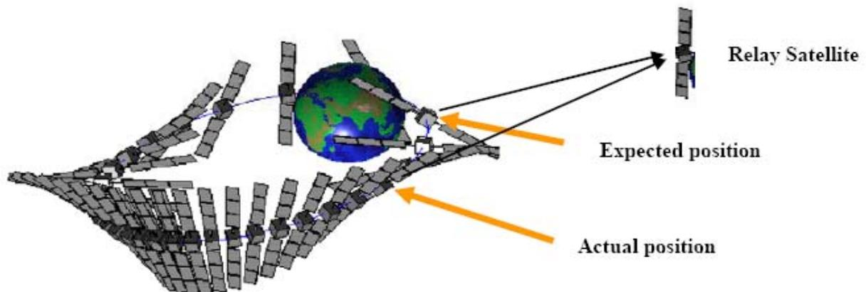
*Figure 6 The use of a relay satellite to eliminate antenna pointing errors*
