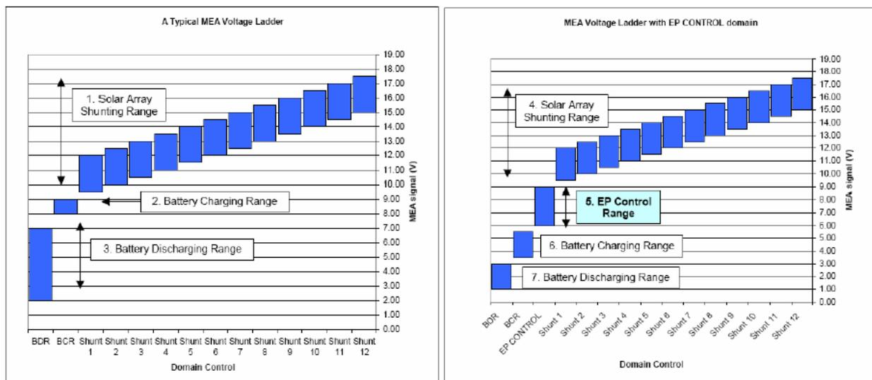
**Figure 3 A typical MEA signal for a regulated power bus (left) and with the addition of an EP control domain for throttling the EP power (right)**
