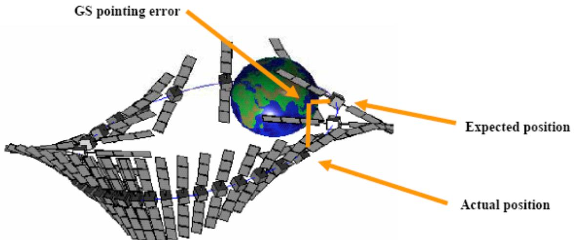
**Figure 1 Schematic of the effect of EP performance variations and unplanned shutdowns on ground station contact (missing impulse shown)**
