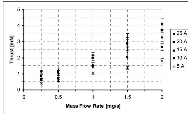
Figure 2. Thrust with xenon as propellant.
