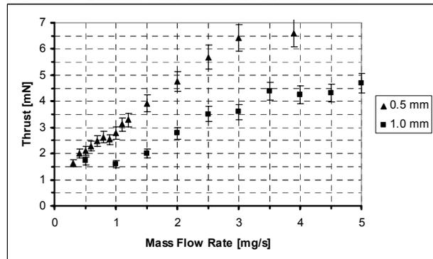
Figure 4. Thrust for two different orifices with argon.
