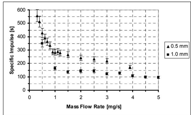
Figure 6. Specific impulse for two different orifices with argon.
