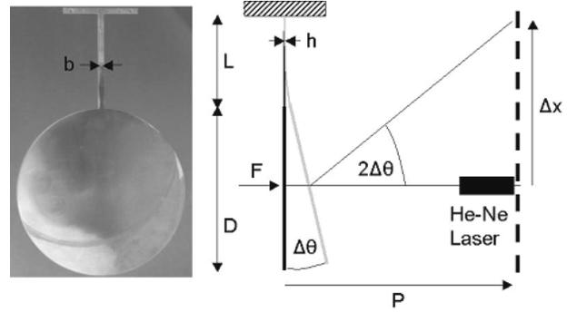
Figure 1. The CBT-LOL thrust measurement system.
