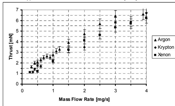
Figure 3. Thrust with different propellants.
