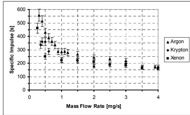
Figure 5. Specific impulse with different propellants.
