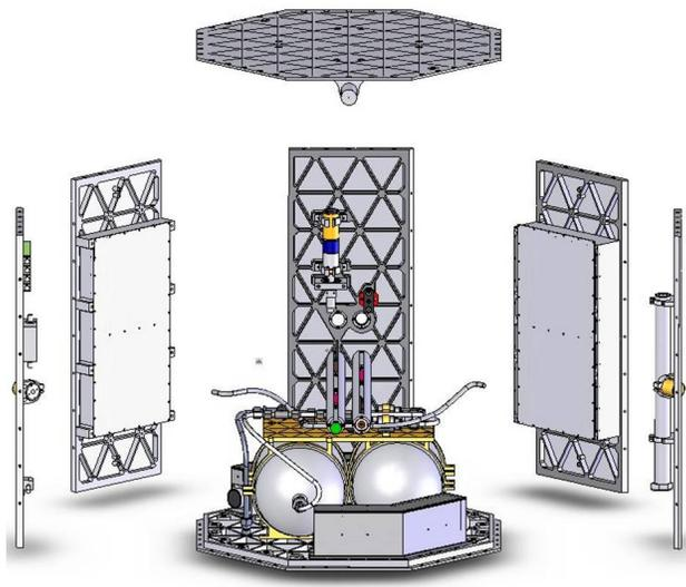
**Figure 5. Exploded view of LionSat**
