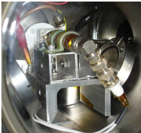
Figure 2. Faraday cup and MRIT in vacuum chamber
